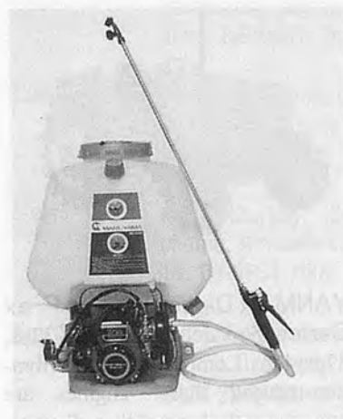
MARUYAMA Portable Power Sprayers MSO55D. Engine: Air-cooled, 2-cycle, output 22.6cc, Pump: Suction capacity 5.1l/mm, max pressure 25 kg/cm 2 . Weight: 8.5 kg.
