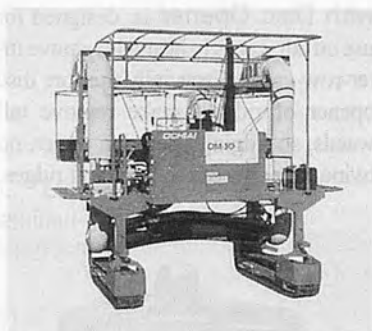
OCHIAI Riding Type Tea Picking Machine OM-30. Full working width cutter bar. Stepless speed control. Water-cooled Diesel engine 28.5PS
