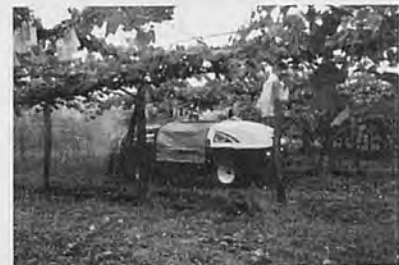
Fig. 7 Microcomputer controlled unmanned air blast sprayer.
