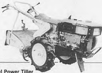
Diesel Power Tiller YT series 4-6hp YTA series 5-6.7hp YZA series 8.5-12.5hp
