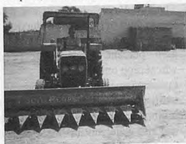
Fig.1 Front view of tractor front mounted vertical conveyor reaper.
