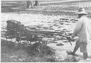
Fig.2 Power tiller attached with two disk ploughs.
