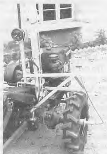
Fig. 3 Wheel revolution counter and fuel measuring device.
