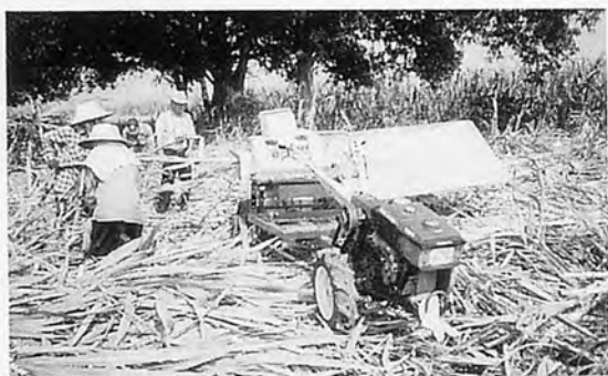
THE BABY LEAF STRIPPING MACHINE (MBC-250C)
