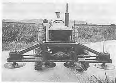
Fig. 2 Pineapple plant dressing machine.
