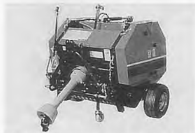
STAR Mini-Roll Baler MRB 0840. Automatic pick-up, rolling and ejection. One bale every 30 seconds, Handy bale size (50cm in diameter and 70cm long). Required tractor horsepower: 18-30 HP.
