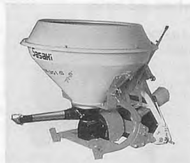
SASAKI Fertilizer Spreader BF-300. The lever type action controls the amount of application with high accuracy. Application width: 10-12m. Hopper capacity: 300l. Required tractor horsepower: 20-50PS.
