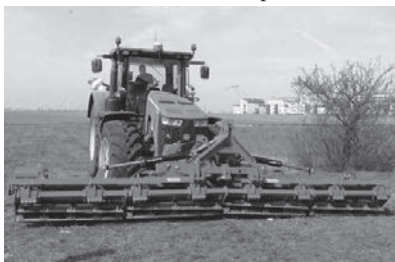
Fig. 3 Example of locally developed and manufactured roller crimper
