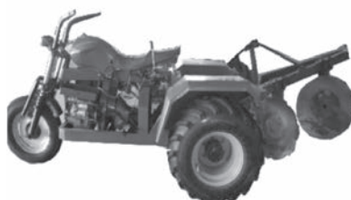
Fig. 2 NCAM developed 30 hp three-wheel tractor (Triketor) with mounted plough
