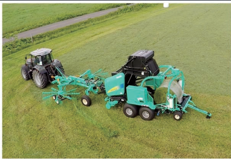
▲ Rake, Bale-wrapper Combination VCW1620
