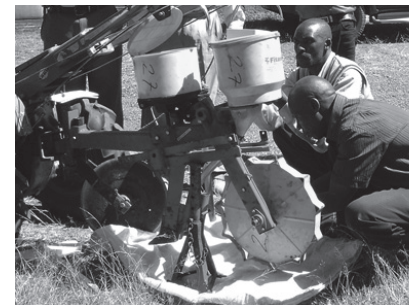
Fig. 5 Calibration of a two-wheel tractor mounted direct planter (Fitarelli, Brazil). (Photo: Brian Sims)
