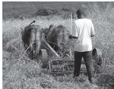
Fig. 4 An animal drawn knife roller for the management of weeds and cover crops. Blades on the roller crimp the plants to desiccate them. (Photo: Brian Sims)
