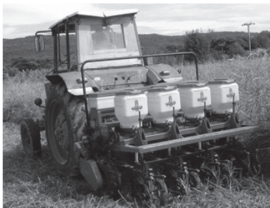
Fig. 3 Tractor-mounted direct planter (Vence Tudo, Brazil). A suitable implement for entrepreneurs to supply CA service to smallholder farmers. (Photo: Brian Sims)
