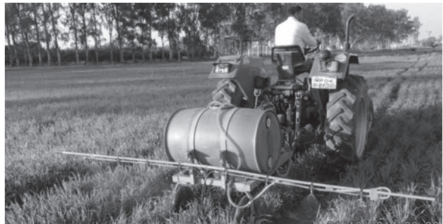
Fig. 2 Sensor based real-time uniform rate spraying system
