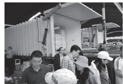
Fig. 8 Mobile precooling system
