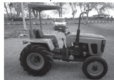
Fig. 3 NCAM developed 45 hp four wheel mini tractor with complete associated implements
