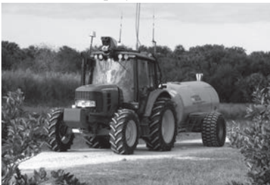
Fig. 1 Unmanned tractor pulling a citrus tree sprayer
