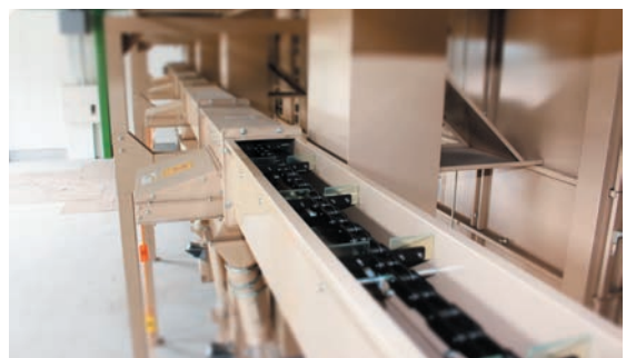
LOADING CHAIN CONVEYOR Power : 10~50t/h
