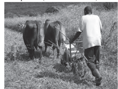
Fig. 2 Animal-drawn direct planter (Knapik, Brazil) with double offset inclined discs to cut through surface vegetation and deposit seed and fertilizer at the required depths in the soil profile. (Photo: Brian Sims)
