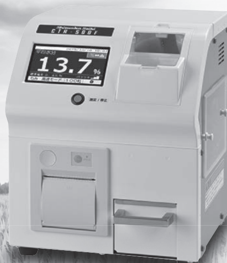
Single Kernel Moisture Meter Model: CTR-500F series
