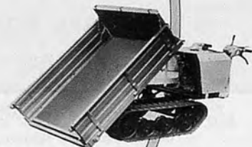
CRAWLER CART SC-6 (SIMPLE TRANSPORT VEHICLE)
