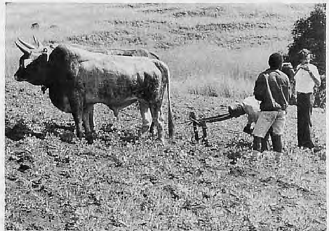
Fig. 3 An animal drawn groundnut harvester in use
