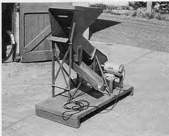
Fig. 4 A power operated winnower for paddy, sorghum and pulses
