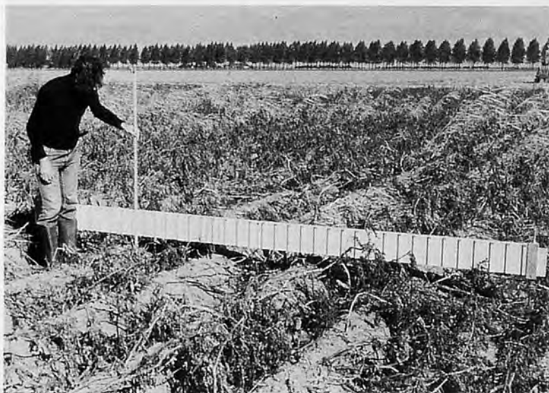
Fig. 2 Measuring the Width of Potato Beds with Relief Meter
