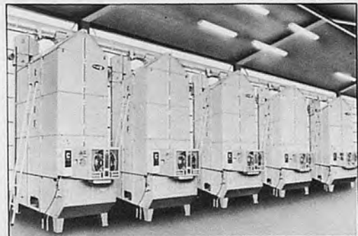
RICECON System—Rice Conditioning System is small-size grain drying and conditioning facilities marked by the separate operation of each dryer and a variety of application.
