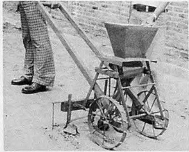
Fig. 2 Pictorial view of three row jute seed drill
