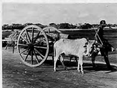
Fig. 3 Orissa bullock cart showing hanged log beneath the cart frame and load on top
