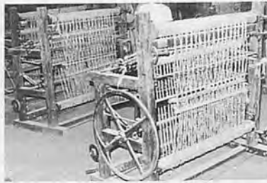
Fig. 5 These are looms for making rice straw bags. A small Korean shop makes them and sells to farmers for off-season enterprises.
