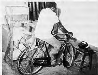
Fig.3 A prototype bicycle operated winnowing machine under test
