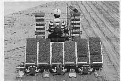
Tractor-mounted rice transplanter (6-rows), at work
