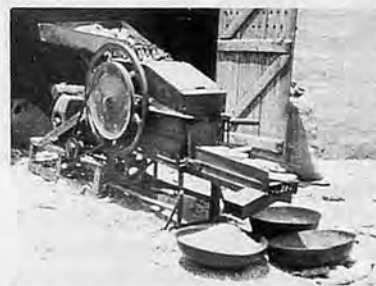
Fig.1 A hand operated maize sheller-grader converted to a power driven unit
