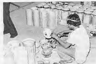
Fig.8 This is a small labor-intensive shop in Indonesia. Back-pack, hand-operated sprayers were being fabricated for local use. Quality control is a problem for these small shops. They need help for the production of durable products to meet the competition of imports.
