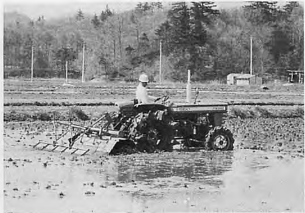
Puddling on submerged paddy field
