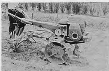
Photo.4 Steel wheel of small tractor for sand dune field.
