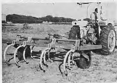
Fig.2 Sweep cultivator for sub-surface tillage
