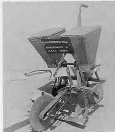
Fig.3 Bukkhar cum ferti-seed drill developed at CAZRI Jodhpur
