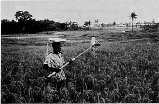
Photo.1 'Micron Ulva' CDA Insecticide sprayer here powered from the sun through a panel of solar cells over the operator's head. Ni-Cad batteries in handles store the excess charge during sunny periods and stabilize the voltage to the motor spinning the spray disc.
