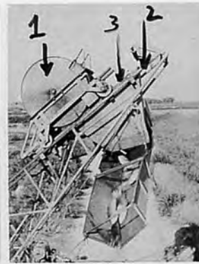
Photo.14 Top end of elevator (1. trolley, 2. pipe rails, 3. elevated rails-on which drum revolves)
