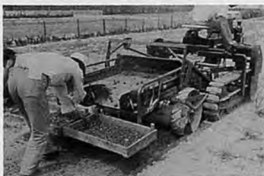
Photo.11 Self-propelled-digging-harvester "Nobel" for Tulip bulbs made in Holland.
