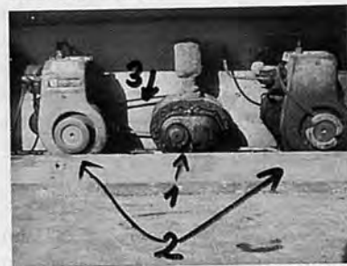
Photo.17 Standard air supply to tank (1. air blower, 2. air cooled petrol engines, 3. V-belt)
