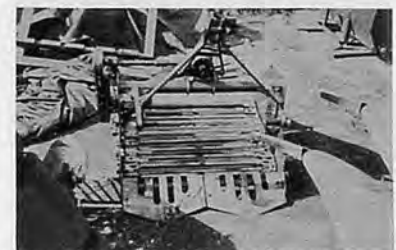
Photo.10 Elevator type digger of large tractor for Tulip bulbs.
