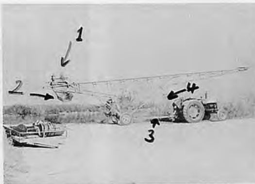
Photo.13 Elevator in transport position (1. trolley, 2. shoot or slide, 3. drawbar, 4. Stay. By folding up the stay, the end of the elevator is lowered in to the pond)
