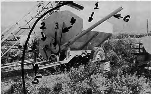
Photo.4 Tractor-driven "Blower" (1. food container, 2. air blower, 3. auger drive, 4. belt-clutch lever, 5. p. t. o.-drive shaft, 6. food blowing pipe)
