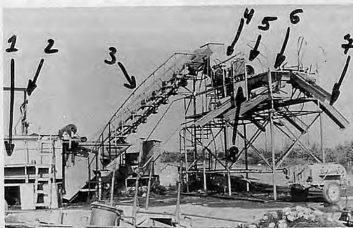
Photo.12 Semi-automatic sector (1. tank, 2. reducing gate, 3. elevator, 4. sorting drums, 5. sorting table, 6. shoots-under which tanks are standing, 8. operating controll)
