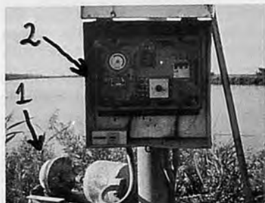
Photo.7 Automatic feeder (1. feeder drive, 2. electronic timer)
