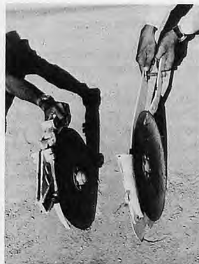
Fig.6 Single and double disc furrow opener for shallow seeding
