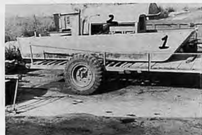
Photo.21 The electric boat on its trailer (1. fiberglass boat, 2. generator)
