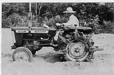
Photo.6 Strake attached rubber tire of large tractor for sandy land.
