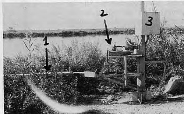
Photo.9 Automatic feeder drive-end (1. perforated pipe and auger end, 2. electric motor and drive, 3. electronic control)
