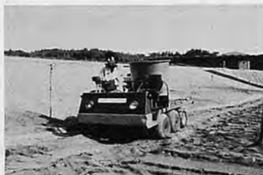
Photo.14 Self propelled six wheels power transporter for sand dune field.
