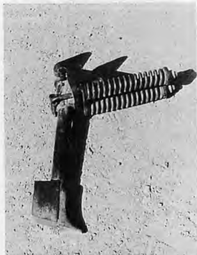
Fig.8 Boot type furrow opener for loose and friable soil
