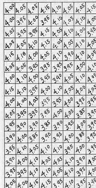
Fig.2 Rod readings after levelling
