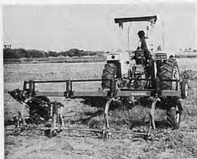
Fig.1 Square-rod weeder for sub-surface cultivation
