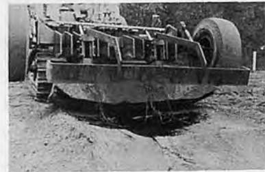
Photo.16 Asphalt injection nozzles of the asphalt barrier machine.
