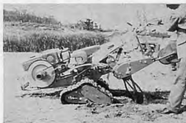
Photo.5 Half crawler and screw tine of power tiller in sand dune field.
