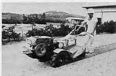
Photo.3 Sinking of power tiller's rubber tires in sand dune field.
