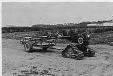
Photo.13 Trailer of small tractor attached half crawler for transportation in sand dune field.
