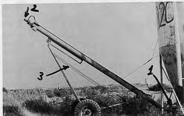
Photo.8 Food auger (1. collecting funnel, 2. hydraulic motor, 3. height adjustment)
