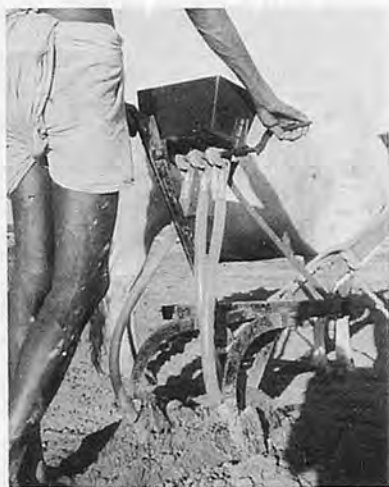
Fig. 5 Line sowing by 3 tine cultivator with Seeding attachment
