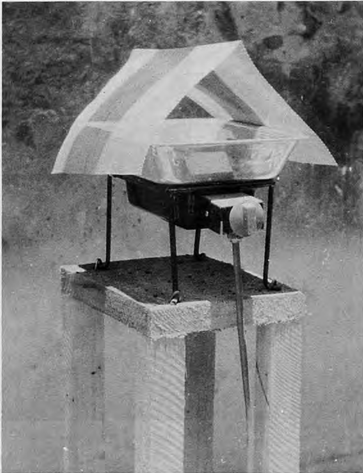
Fig.2. Gas burning infra-red heater (note: the write-mesh protective cover avoids incineration of falling cocoa particles.)
