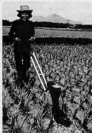
Fig.4. Two-row liquid band applicator in operation at 3 days after transplanting.
