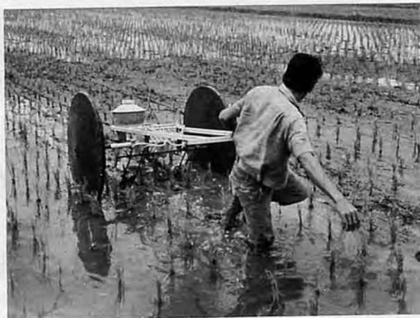
Fig.2. Four-row peristaltic pump liquid injector.
