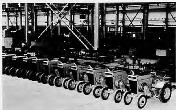
Fig.1. Pakistan's first 10-horsepower tractor M-10 under production.
