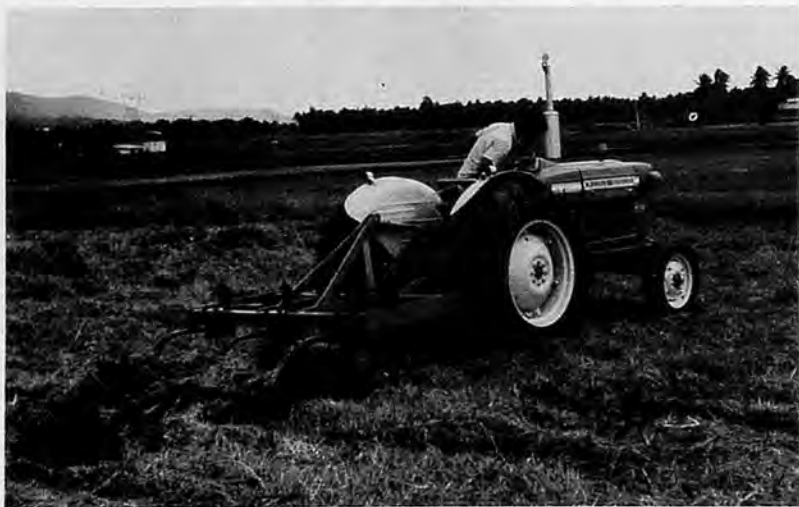
Fig.2. Howard chisel plow for breaking the hardpan and for inter-row cultivation.
