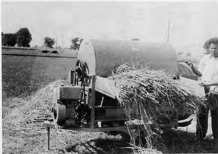
Fig.3. The IRRI thresher is now in regular commercial production in Pakistan. This unit is manufactured by Lahore Engineering Foundry Limited (Lefo).
