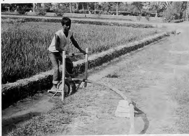
Fig.4. The locally produced diaphragm pump is being used at Rice Research Institute, Kala Shah Kaku, Lahore, Pakistan.
