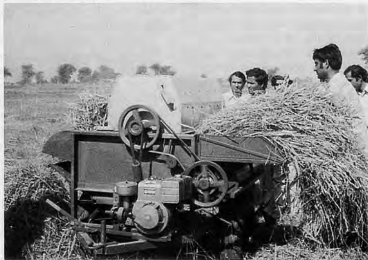
Fig.2. Field testing of IRRI design axial flow rice thresher at Rice Research Institute, Kala Shah Kaku, Lahore. The satisfactory performance on local condition has been achieved after incorporating some modification in the original design.
