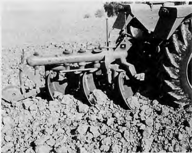
Fig.5. Deep ploughing by disc plough (or by mouldboard plough) adversely affects moisture conservation.
