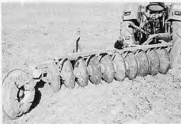
Fig.7. A disc-tiller or one-way tiller—an economic and widely used tillage tool for dryland farming is yet to be popularised in Iraq.
