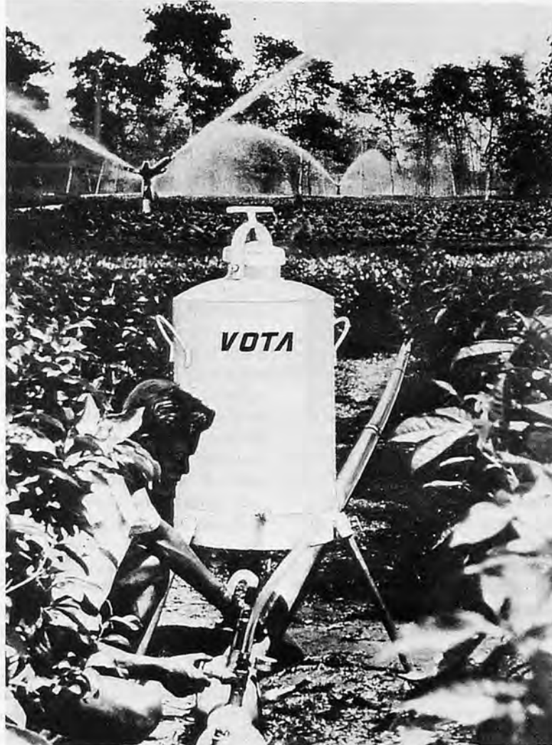
Photo.1. Application of Fertilizer Through Sprinkler Irrigation System
