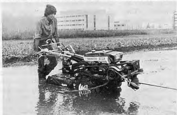
Fig.1. A view of the braces and frames used to support the gear box, extended PTO shaft and all other accessories.
