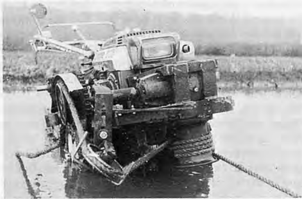
Fig.2. A closer look at the winch assembly showing the change in direction of the rope by using the pulley arrangement.
