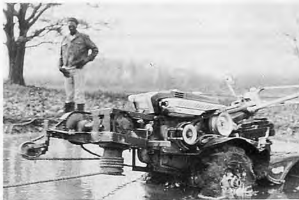
Fig.8. The front end of the tractor was lifted when the winch system was used.
