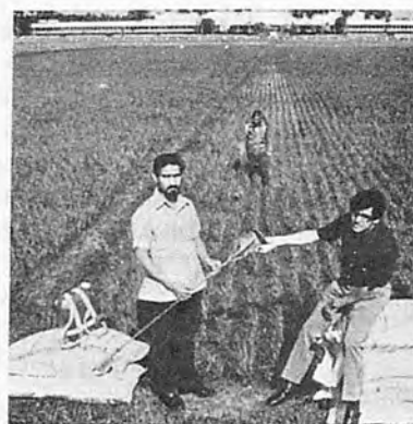
Fig.4. Engineers are working with agronomists and entomologists to develop and test simple, inexpensive implements to speed chemical placement into the root-zone. Holding a prototype of a new liquid urea pesticide applicator are: right, Amir U. Khan, agricultural engineer; and left, Nestor Navasero, senior research assistant. The applicator is being demonstrated in the background.
