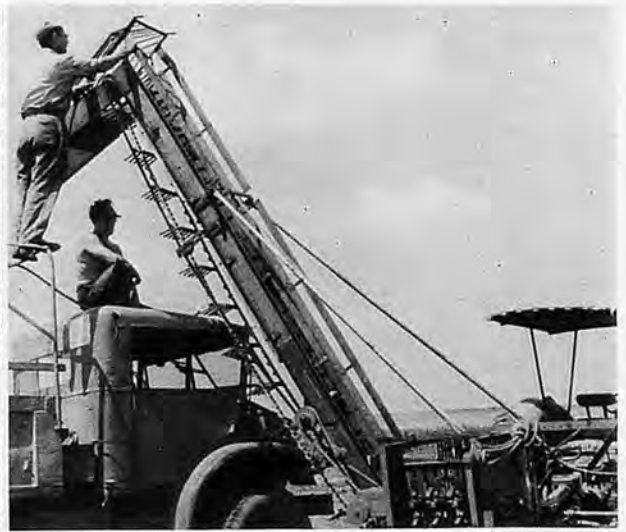
Photo.2. Maayan Zwi. A one-row sugar beet harvester which was bought as a standard machine but completely re-constructed and adapted to local conditions, lifting-cleaning-loading onto truck.
