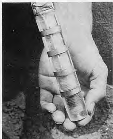
Fig.2. Researchers at Riverside have also developed a single-probe device for taking spot readings of salinity. That device has the four electrodes inlaid in a single shaft (the four metal rings in the photo above, PN-4109), which can be inserted in a standard soil sampler hole (below, PN-4110)
