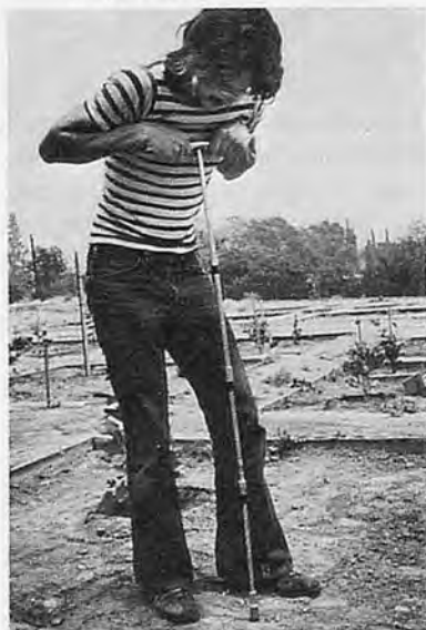
Fig.2. Researchers at Riverside have also developed a single-probe device for taking spot readings of salinity. That device has the four electrodes inlaid in a single shaft (the four metal rings in the photo above, PN-4109), which can be inserted in a standard soil sampler hole (below, PN-4110)
