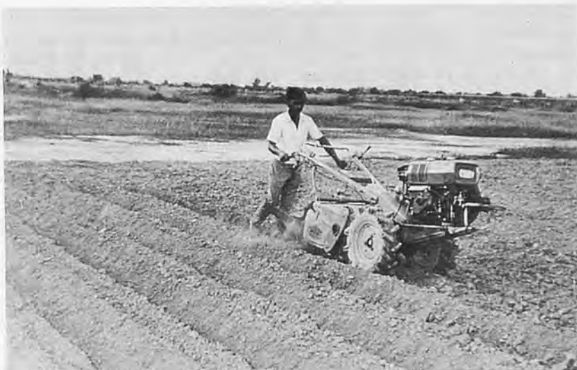
Photo.2. Ridging with locally manufactured power tiller.
