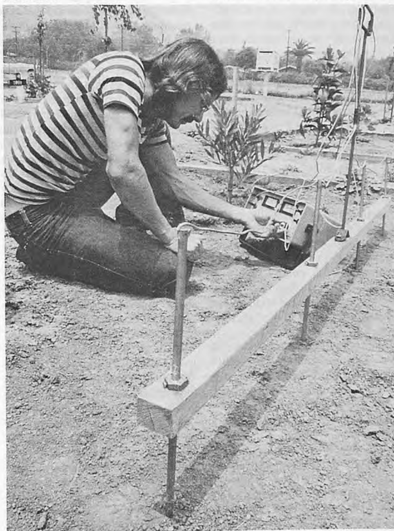
Fig.1. Using a new four-electrode device, scientists are able to make quick, easy soil salinity measurements in the field. Soil scientist Robert J. Prather adjusts a meter used to measure the resistance of electrical flow between the inner pair of electrodes (PN-4108)
