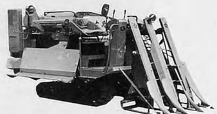
model RC-901 Engine=11~15HP Cutting wide=900mm 3row cutting Efficiency=40~70minutes/10ares
