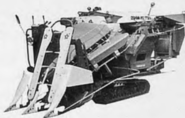
model RS-701 Engine=8~11HP Cutting wide=700mm 2row cutting Efficiency=60~90minutes/10ares
