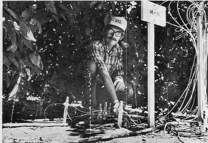
Fig.6. Chemist Robert Ingvalson inspects the drip system and tensiometers under a tree. While it is called drip, water actually squirts at 1-foot intervals from a tube coiled around the base of the test tree. The tensiometers measure soil-water suction at 15, 30, 45, and 60 centimeters (cm) beneath the trees. Other tensiometers set at 30 cm under the trees sense when a predetermined “dryness” is reached and activate the drip system for that particular test area (0874R1408-14).
