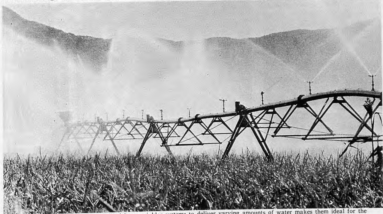
Fig. 1. The ability of electrically driven sprinkler systems to deliver varying amounts of water makes them ideal for the ARS research being conducted in the Grand Valley to determine the effects of salinity on irrigation management along the Colorado River Basin and on other arid lands where irrigation is required (0874R1403-16).
