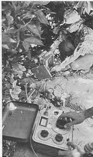
Fig.8. Dr. Ingvalson checks a control point which can be set to deliver different amounts of irrigation water to different areas while Dr. Wood takes a salinity reading from an underground sensor (0874R1409-30).
