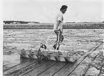
Fig.8. Paddy seeder operated on a properly drained puddled field
