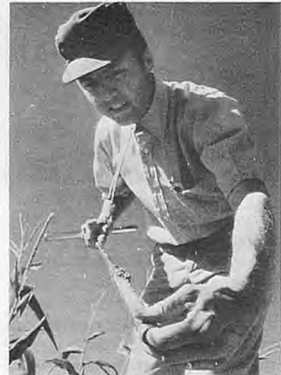
Fig.4. Soil samples are taken frequently for comparison with readings from equipment buried in the test field. Biological technician Gordon Fischbacher takes a sample that will be analyzed for soil moisture, salinity, and CO 2 content (0874R1399-21A).
