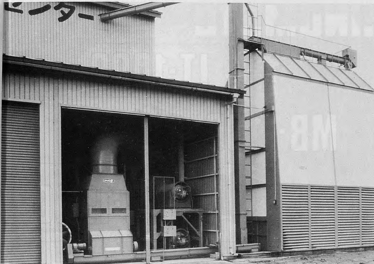
Picture above ISSHIN-GO FDA System Equipment set indoors (left) shows preliminary fluidized-bed dryer. Equipment outdoors (right) shows moisture control finishing dryer.
