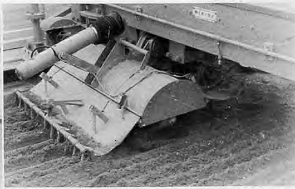
Photo 8. Rotary tiller simultaneously conducting tilling, leveling and furrowing
