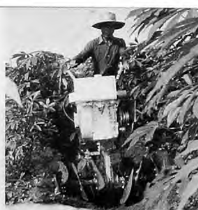
The same "pedestrian tractor" re-developed here for throwing up high ridges for the growing of tapioca ( Manihot Utilisima ). Growth is much improved, weeds controlled entirely and lifting of tubers facilitated. Special rotors were designed for ridging simultaneous with cultivator.
