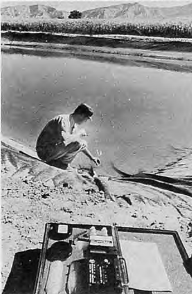
Fig.5. Mr. Fischbacher takes a salinity reading from the reservoir which feeds the sprinkler system. The 27-acre experimental plot is in the background (0874R1405-7).
