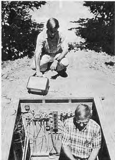
Fig.7. Soil scientist James Wood watches as Dr. Ingvalson examines vacuum regulators which collect moisture through tubes located at a 4-foot depth below the entire test area. The moisture is analyzed for volume and chemical content (0874R1407-34).
