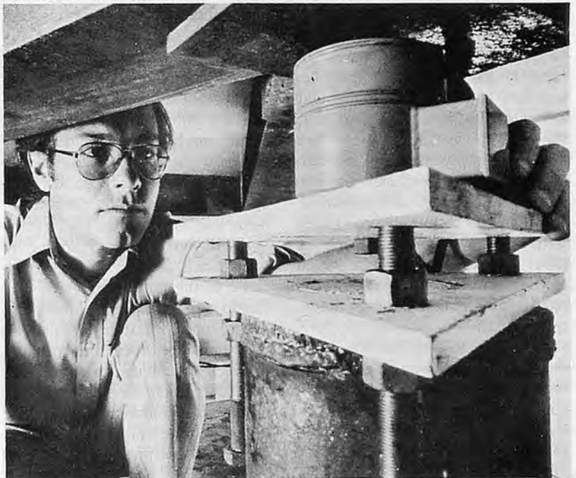
Fig.9. Lysimeters buried beneath the test plots check moisture use of the plants and underground water flow. Agricultural engineer Dennis Kincaid checks one of the three load cells that, despite being under 10 tons of soil, can detect a "heavy dew" (0874R1401-1).
