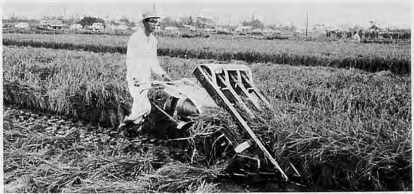
Fig. 15. Development of binder begins at three row cutting in 1966, after being miniaturized year by year, at present the main is one row cutting binder.
