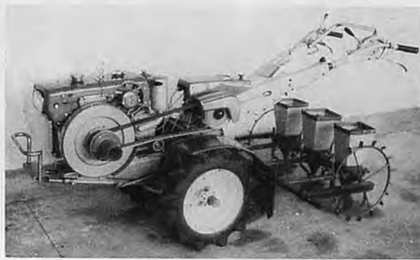
Fig.6. Two wheel tractor drawn 3 row seeder for paddy. (Could be used to seed other crops : maize, soyabeans, pulses, sorgham, groundnut, etc.)
