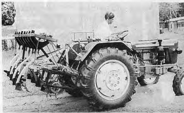
Fig.5. Tyne tiller mounted 8 row paddy seeder. (Could be used to seed other crops : soyabeans, green gram & cowpea)
