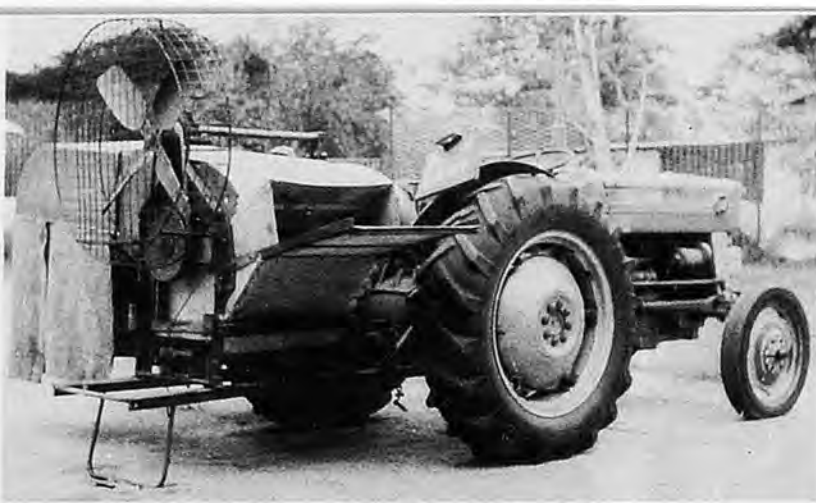
Fig.7. Four wheel tractor Power Take off driven thresher for paddy (Could thresh soyabeans and sorgham also)
