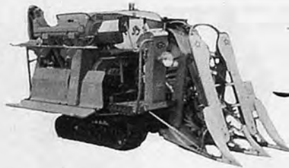
model RS-701 Engine=8~11HP Cutting wide=700mm 2row cutting Efficiency=60~90minutes/10ares
