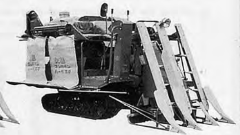
model RC-901 Engine=11~15HP Cutting wide=900mm 3row cutting Efficiency=40~70minutes/10ares
