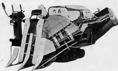
model RS-600 Engine=7~9HP Cutting wide=650mm 2row cutting Efficiency=80~120minutes/10ares
