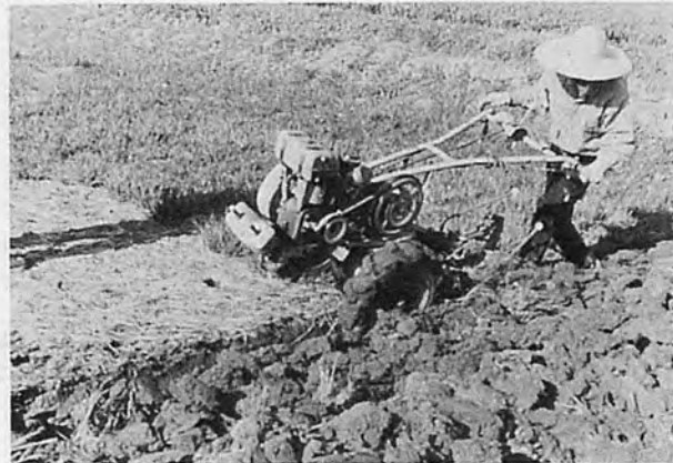
Photo No.2 Spring season cultivation in paddy field by 3 hp power tiller with a reversible Nippon plow.
