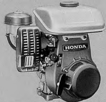
G42 / G65 General Purpose Engines 170cc (G42) or 240cc (G65) gasoline engine. Output: 4.5hp/4,000rpm (G42); 6.8hp/4,000rpm (G65). Weight: 18.3kg (G42); 29.1kg (G65).
