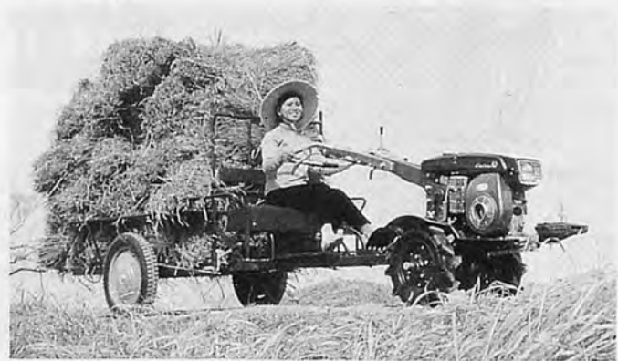
Fig.16 Pipe-Frame trailer with a 6.6ps hand tractor (source; Trade and Industry of Japan , JETRO, 1968, p. 128)
