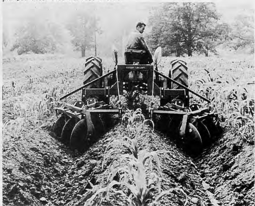
Figure 3. Border disc attachment for constructing and maintaining ridges and furrows.
