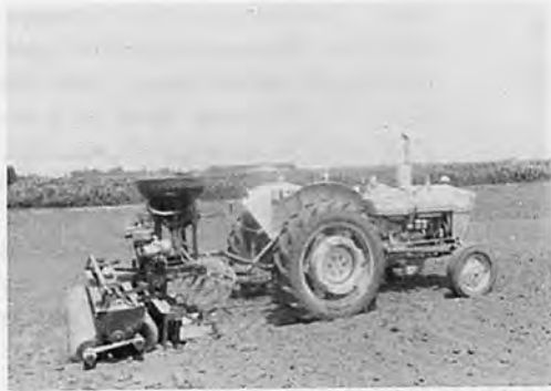
Fig.8 soil-incorporation of herbicide by tractor-mount-type-granule-applicator
