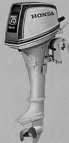
Outboard Engine 7.5bhp gasoline. 4-stroke OHC in-line twin cylinder engine. 149cc (9.1cu.in.) displacement. 13 liter (3.4US gal, 2.9 Imp. gal.) separate tank capacity. Weight: S Model 27kg (60lb); L Model 28.9kg (64lb)
