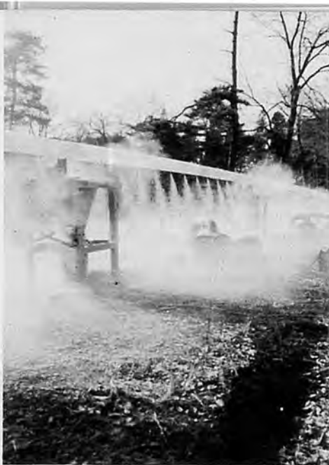
Test of discharge rate of dust from the pipe of travelling power duster
