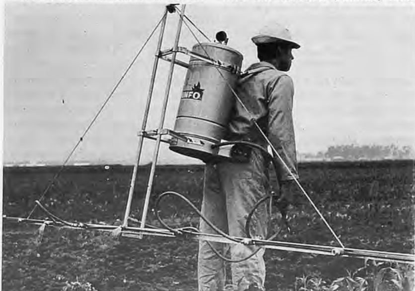
Fig. 1 A tailboom fitted to a compressed air, knapsack sprayer permits the operator to continually move away from the area just sprayed.
