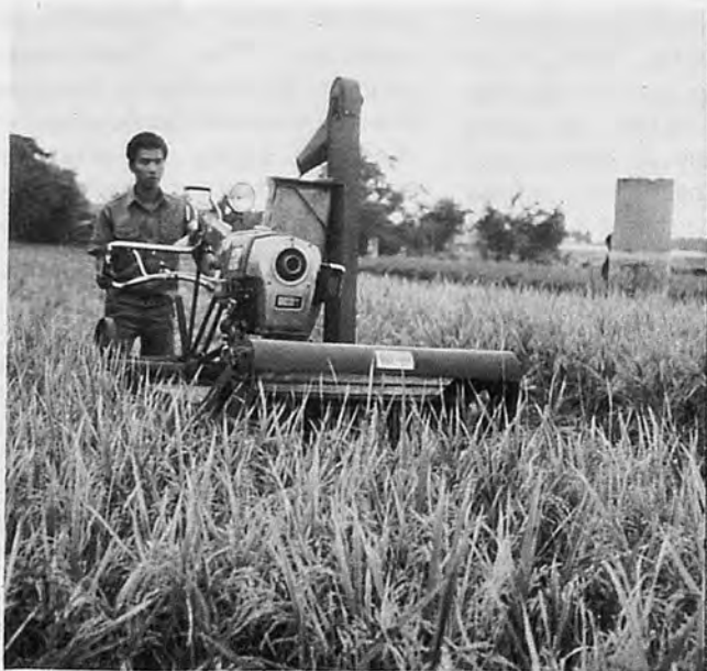
STRIPPER HARVESTER: This four-row machine can harvest paddy in the field without cutting plants. Since straw is not handled through the machine, it is light and compact. Combined scattered and unthreshed grain losses of only 1.5 percent have been obtained in some tests with this stripping principle in a laboratory machine. Further development work is underway.
