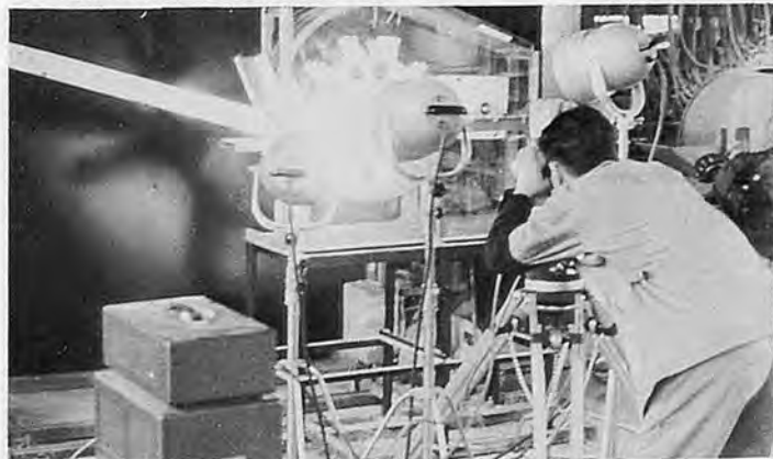
Analysing of threshing mechanism by fast motion camera
