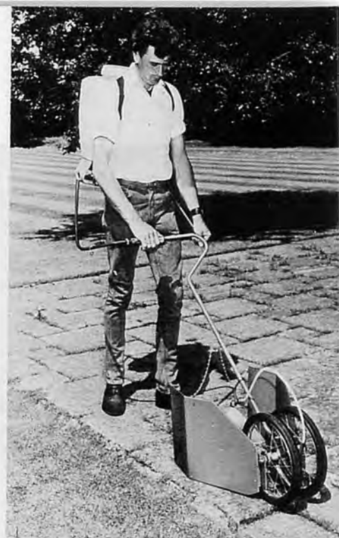
Fig. 2 Guards mounted on wheels limit spray.
