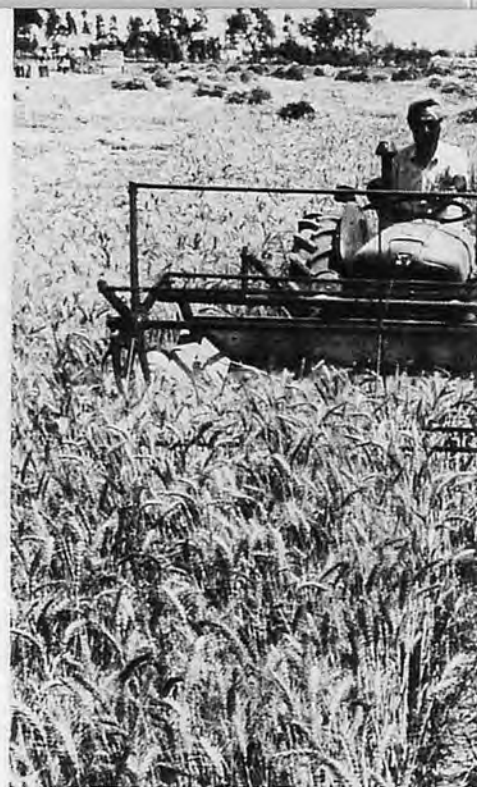
Fig.4 A 1.8 metre Cutter bar Tractor Front Mounted Punjab Agr. University, Ludhiana for Wheat
