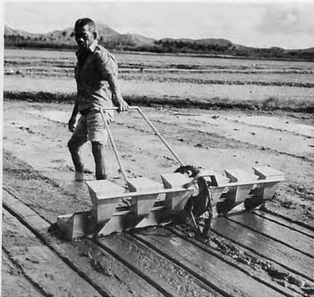
MULTIHOPPER PADDY SEEDER: This is a low-profile seeder with six independent hoppers for seeding pregerminated paddy on puddled soils. No cut-off mechanism is used to meter the seeds which minimizes damage to the sprouted seed. The machine has been released for commercial production in the Philippines and is expected to sell for US$40.00.
