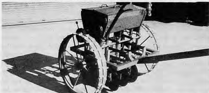
Fig.2 A Typical 3-Row Bullock Drawn Seed-cum-Fertilizer Drill for Sowing Wheat, Barley, Gram, Peas etc.
