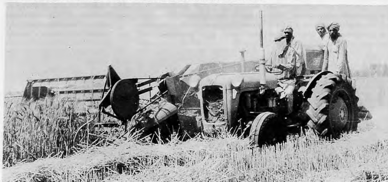
Fig.7 Tractor Side-Mounted Vicon Combine with 1.5 Metre Cutter Mumber about 200 in Northern India. These are Being Manufactured in India
