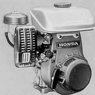
G42/G65 General Purpose Engines 170cc (G42) or 240cc (G65) gasoline engine. Output: 4.5hp/4,000rpm (G42); 6.8hp/4,000rpm (G65). Weight: 18.3kg (G42); 29.1kg (G65).
