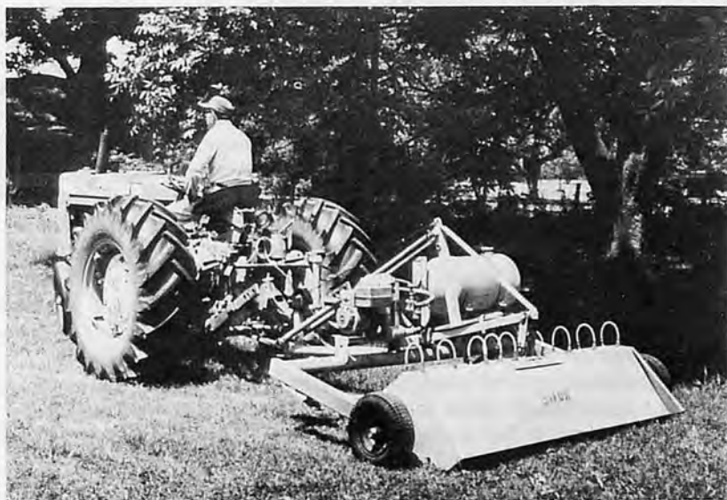
Fig. 6 Low volume spray is ejected under the hood of this trailed sprayer.
