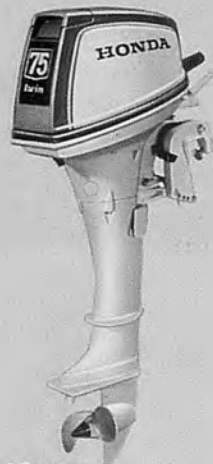
Outboard Engine 7.5bhp gasoline. 4-stroke OHC in-line twin cylinder engine. 149cc (9.1cu.in.) displacement. 13 liter (3.4US gal, 2.9 imp. gal.) separate tank capacity. Weight: S Model 27kg (60 lb); L Model 28.9kg (64 lb)
