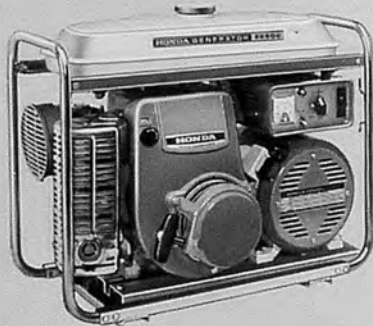
E2500 Portable Generator 6.8hp gasoline engine. 120-240V 2500W AC and 12/24V 100W DC. Weight: 79kg.
