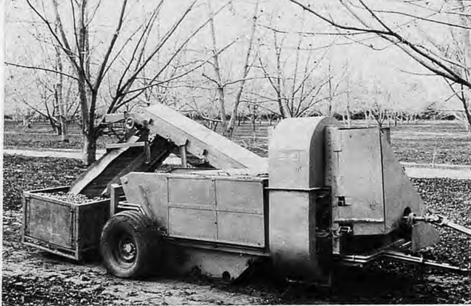
Fig. 5 A prototype of collecting machine for pecan nuts
