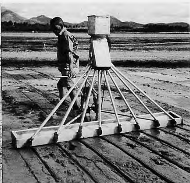
SINGLE HOPPER PADDY SEEDER: This machine can sow pregerminated paddy in rows on puddled soils. Five to seven hours are required to seed one hectare. The machine has a single wheel to facilitate transport on narrow field levees and to provide the motive power for the metering mechanism. It is commercially produced and sold for about US$45.00 in the Philippines.
