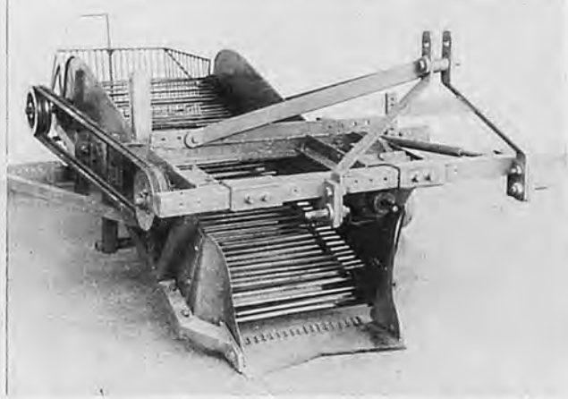
Fig.6 A Single Row Potato Elevator Digger Developed at The P. A. U. Ludhiana
