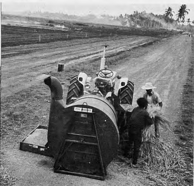
TRACTOR PTO THRESHER: This machine has been developed for custom threshing of rice and other grain crops in Asia. It can thresh dry as well as freshly harvested crop. The thresher is mounted on a tractor three-point linkage and is light enough for lifting with standard hydraulic systems. This feature provides easy field maneuverability. Threshing output of 1.5 tons per hour has been obtained.
