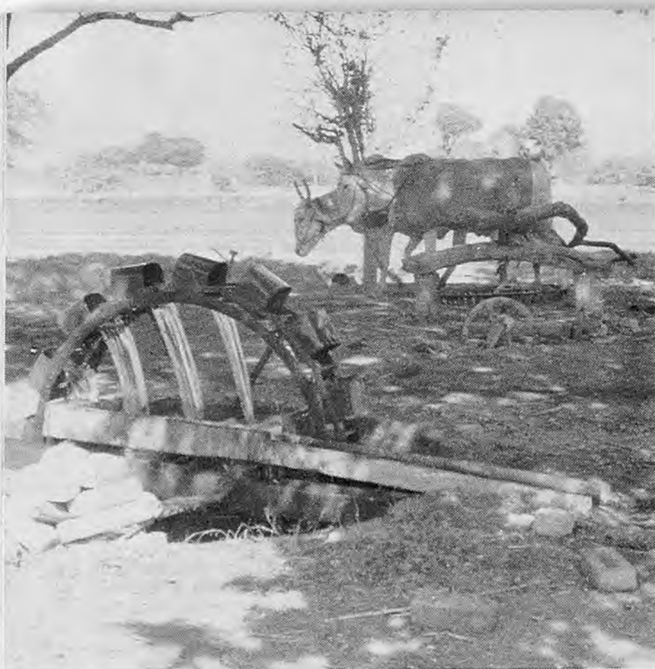
The Persian wheel is the most effective instrument for irrigation before the introduction of motorized energy. The Persian wheel is most common in Northwestern and Northern India. It can be utilized only, if the groundwater reaches a high level.
