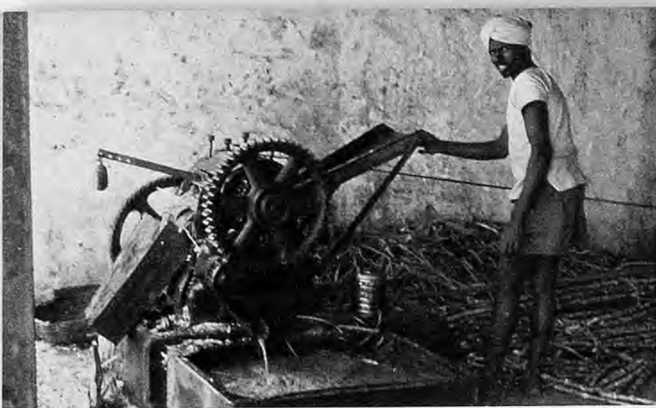
Processing of sugarcane. The cane is crushed and pressed with a motorized cane-crusher. The juice is cocked and slowly condensed into gur, a semirefined, yellow-brown raw sugar, which is marketed and quoted in the markets.
