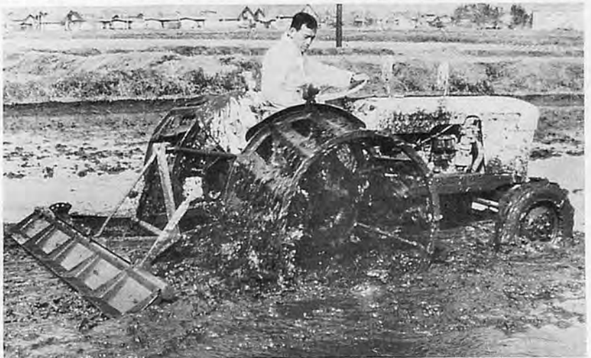
A DB 780 fitted with special cage wheels levelling a paddy field
