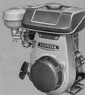
G41/G65 General Purpose Engines 171 cc (G41) or 240 cc (G65) gasoline engine. Output: 4.5 hp at 4,000 rpm (G41); 6.8 hp at 4,000 rpm (G65). Weight: 17 kg (G41); 29.1 kg (G65).
