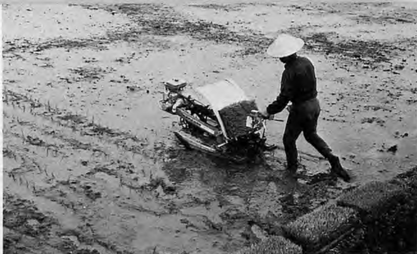
A power rice transplanter of early seedling with soil type shown on this picture is most popular at present (Kubota SPS-28)
