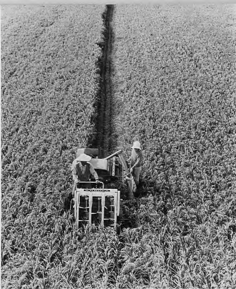
Central harvesting work by a three-row type combine which is most efficient among all head feed combines (Kubota HT90)
