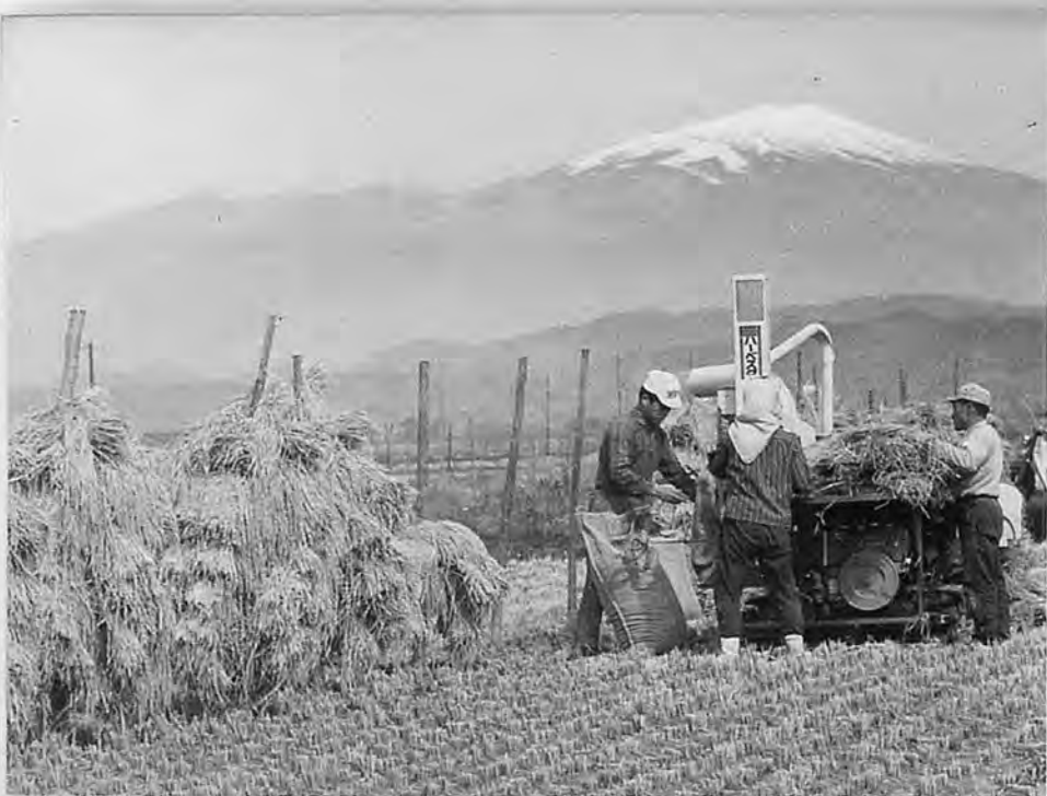
It's a charming point of a self-propelled automatic thresher "to be able to thresh paddy while traveling freely on paddy field" (Konma MT)
