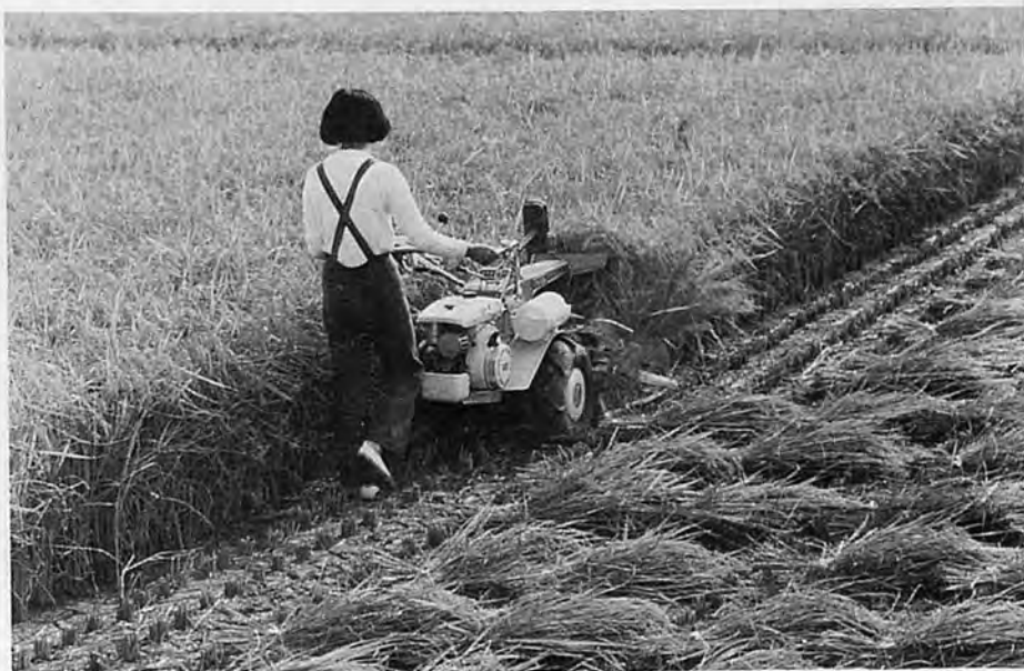
Even a woman can operate conveniently a one-row type binder (Iseki RS-250)
