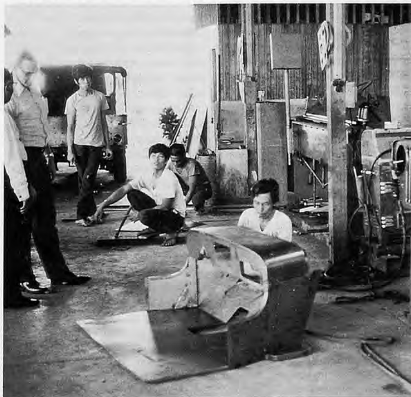
Small factory for jeepny production in the Philippines. 11 people make 5-6 units of jeepny body for a week.
