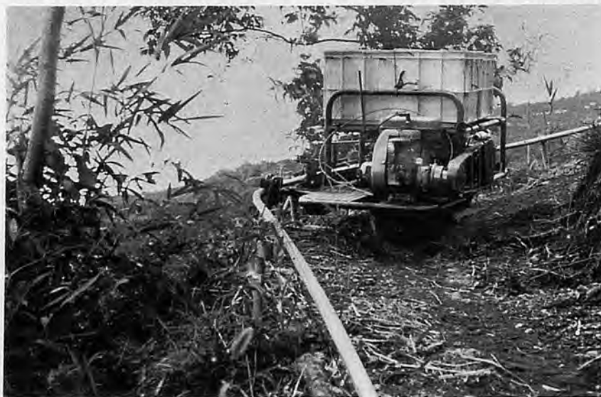
This two-wheel type transporter runs along guide rail (Wamulass Line carrier DW-10)
