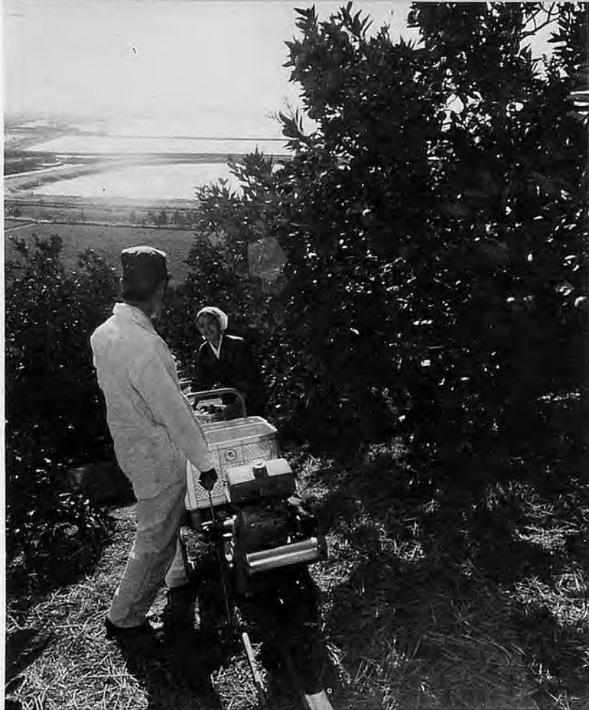
Many horticulturists utilize a monorail car which they can start and stop as they like it ( Nikkari Mono-Rack M-70 )
