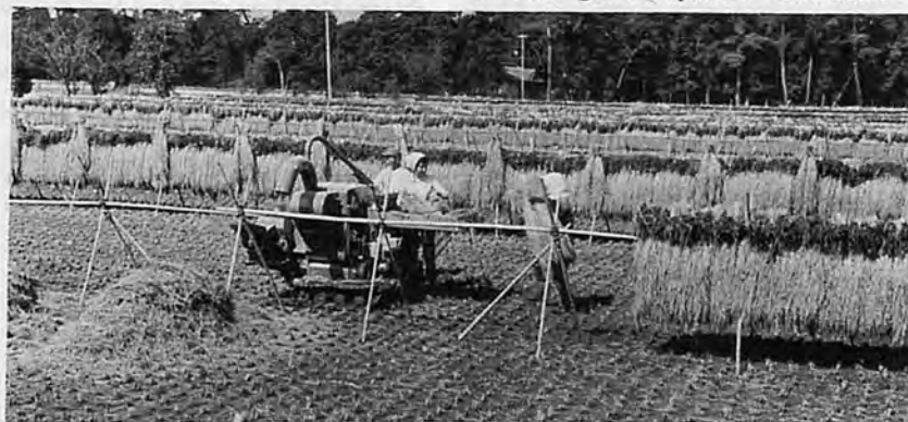
A self-propelled automatic thresher, which can thresh rice while traveling on paddy field, reduces labour for farm work (Yanmar PTC)
