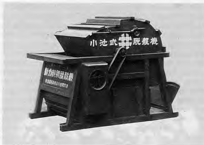
Threshers made the basis of farm mechanization firm in Japan. This thresher is almost wooden
