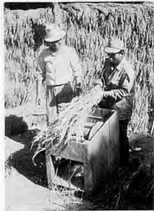
Fig. 8 Japanese type pedal thresher made in Laos. As it mixes up much dropped rough rice and chaffs, a wind fan fox separating must be attached, at the same time. They are not patient enough to continue treadle work for hours. It costs them 9500 kip. It is made by utilizing secondhand bicycle etc.
