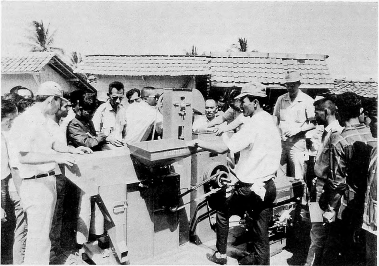
Demonstration of a hulling and pearling equipment in West Java. (Though small, this equipment can deal with 3 ton a day)
