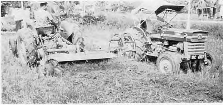
Fig. 3 Rotary tillers working in a moist field. Note cage wheels on one tractor.
