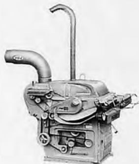
Highly efficient chain feeding thresher — super drawing type Easy to operate with the under-chain method.
