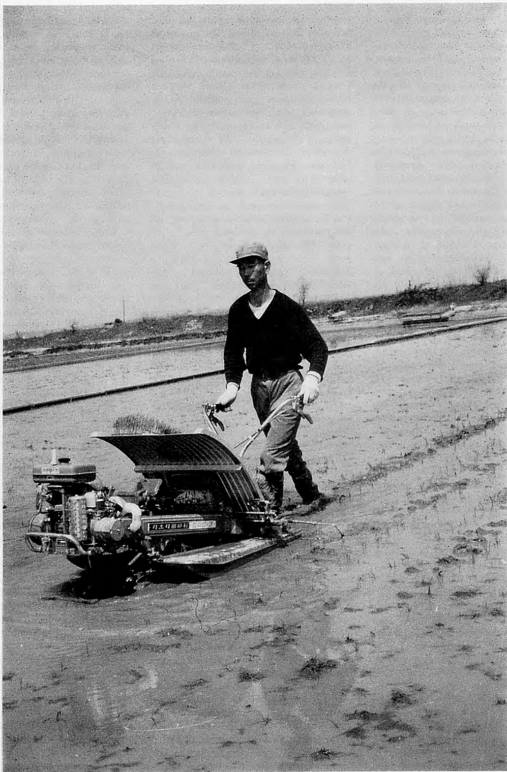
Rice transplanting machines—a terminal of rice crop mechanization are spreading in Japan
