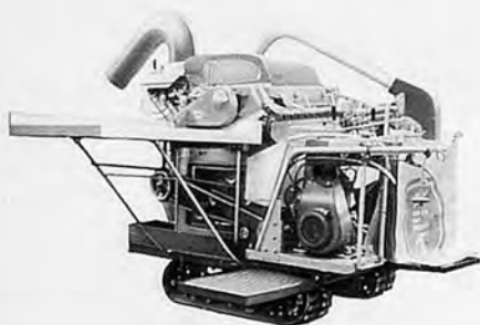
Self-propelled chain feeding thresher — mini-type Light and compact self-propelled thresher.
