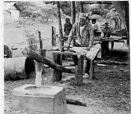
Fig. 9 Old wooden burr used in Laos. It is used for rice pearling. It takes 3 children 1~1.5 hours to mill 10kg of rough rice.
