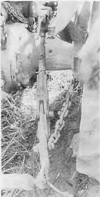
Fig. 5 Heavy auxiliary sway chain. Note many welded reinforcements on lower draft link and connecting rod. The use of disc implements restrained by tight sway chains cause many failures of draft and lift linkage parts.
