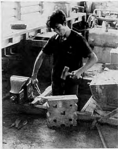
Fig.11 Practice of smithery in a corner of a repair shop. He is tackling with a used blade of a power tiller.
