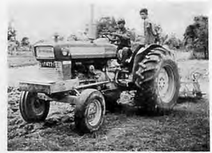
Fig. 1 Four-wheel tractor of the 50- to 70-hp type commonly used in tractor contractor operations in Thailand and Malaysia.
