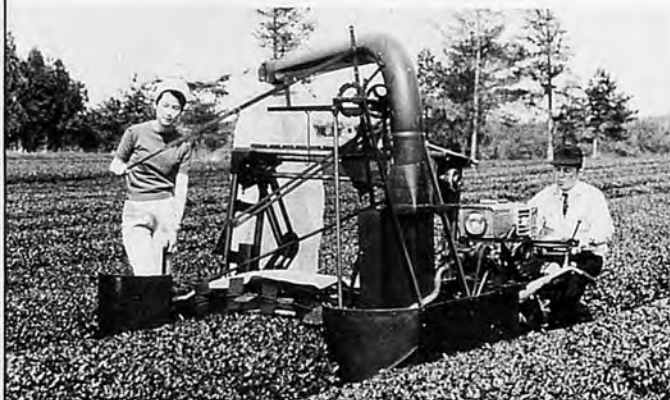
AUTO. TEA-LEAF PILING & TEA-FIELD SUPERVISING MACHINE. ■ UCHIDA'S "KIRISHIMA" PAT.
