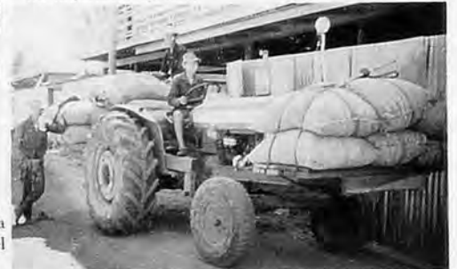
Fig. 8 Tractor with front and rear transport platforms fully loaded. Such loads cause frequent failure of front wheel bearings.
