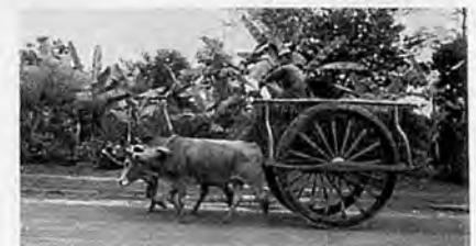
Fig. 10 Ox-cart used in Laos. It is serviceable in waters of 60~70cm deep and coves. It costs 70,000 kip.
