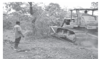
Fig. 3 Model D8 in operation pushing and felling down of vegetation
