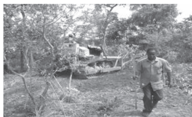
Fig. 2 Model D7 in field operation pushing and felling down of vegetation
