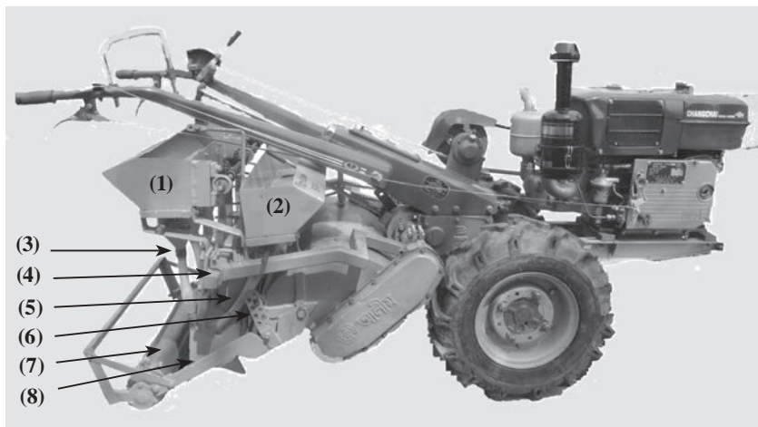
1: Seed box, 2: Fertilizer box, 3: Seed delivery tube, 4: Toolbar frame 5: Fertilizer delivery tube, 6: Depth controller, 7: Press roller, 8: Furrow opener
