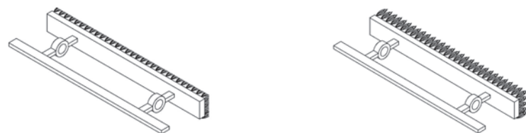
Fig. 6 Different types of pulping Beater a. with shorter beater length b. with longer beater length
