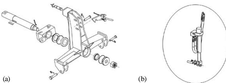
**Fig. 2** a) Implement connecting frame for mounting to the tractor three point hitch
