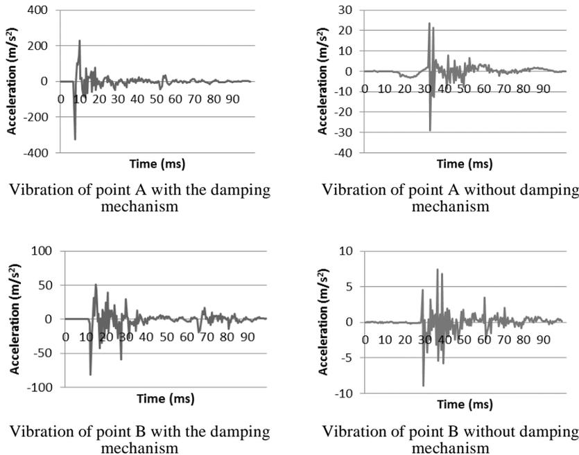
Fig. 10 Examples of vibration signals picked up at points A and B of the plow frame with and without the use of the damping mechanism
