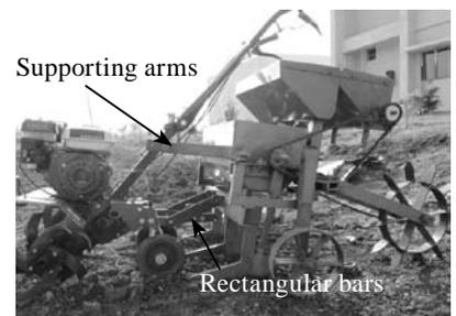
**Fig. 5** Mounting of groundnut planter to the power weeder
