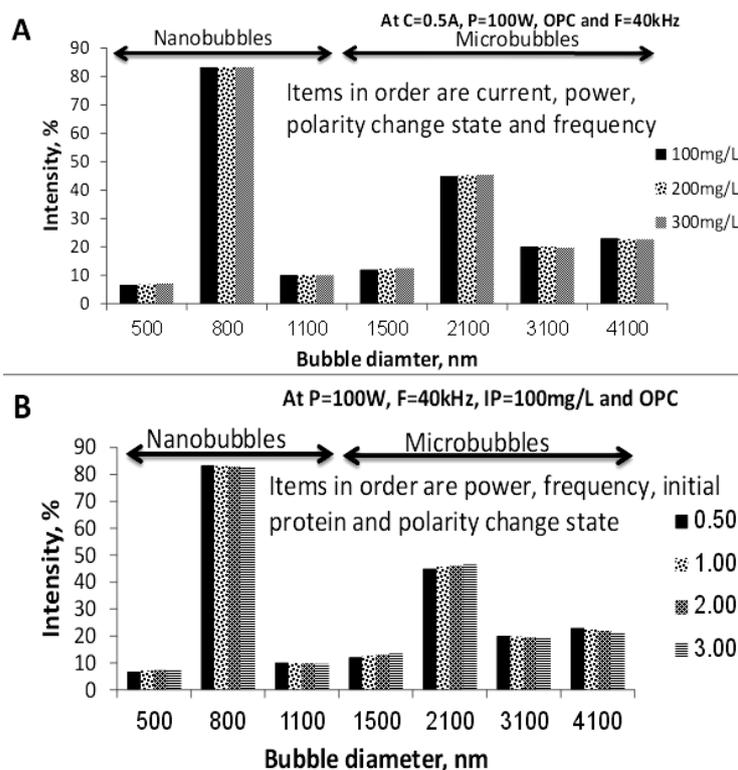
**Fig. 3** The effect of initial protein concentration (A) and electrical current (B) on bubble size distribution generated as microbubbles or nanobubbles by a combined electro-coagulation with ultrasonication for bubble generator
