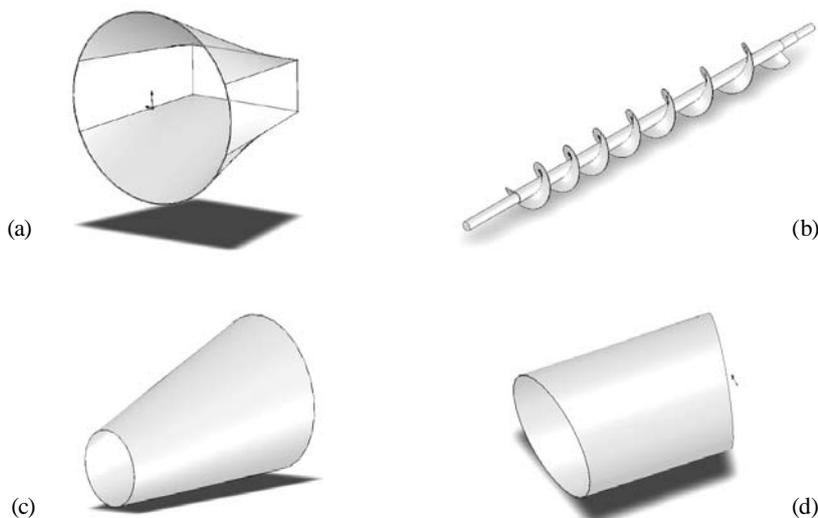
**Fig. 1** Special shapes (a) circle to rectangle transition, (b) variable pitch auger, (c) oblique cone and (d) segmented bend.
