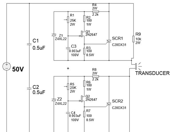
**Fig. 1** Electronic circuit of ultrasonic generator with output of 200W and dual frequencies of 40 and 60 kHz
