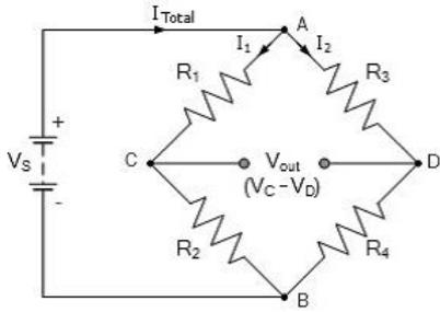
**Fig. 8** Wheatstone bridge circuit diagram in dynamometer
