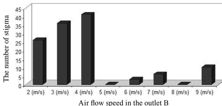
**Fig. 7** The relationship between the number of stigma that exit from outlet B and air flow speed in the outlet B
