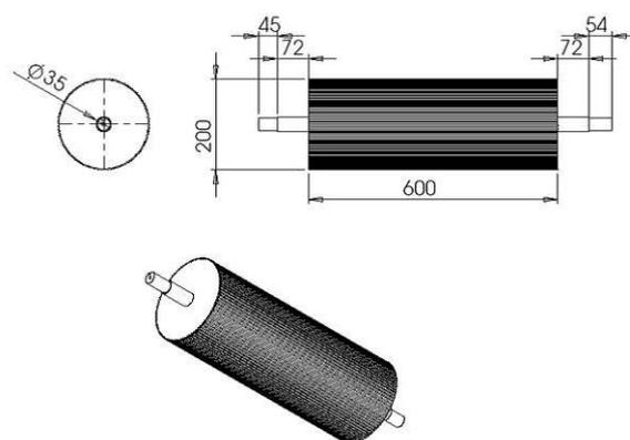
**Fig. 6** Configuration of Output roller
