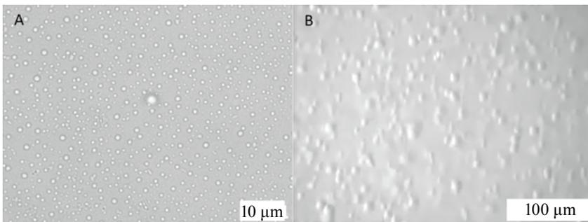
**Fig. 6** Captured photos by optical microscope with magnification up to 1,000X (A) and by a digital microscope (B) connected to laptop with USB connection with magnification of 500X for real time monitoring
