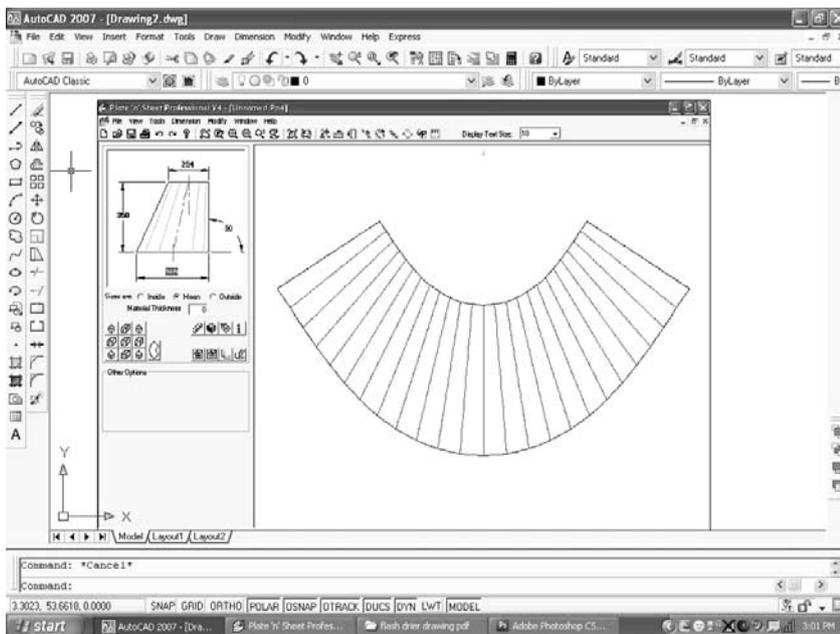
**Fig. 5** Screenshot of Plate'n'sheet template inside AutoCAD
