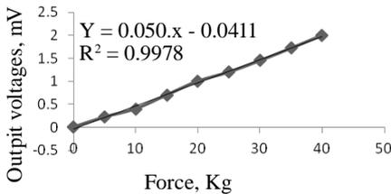
**Fig. 16** Calibration of dynamometer
