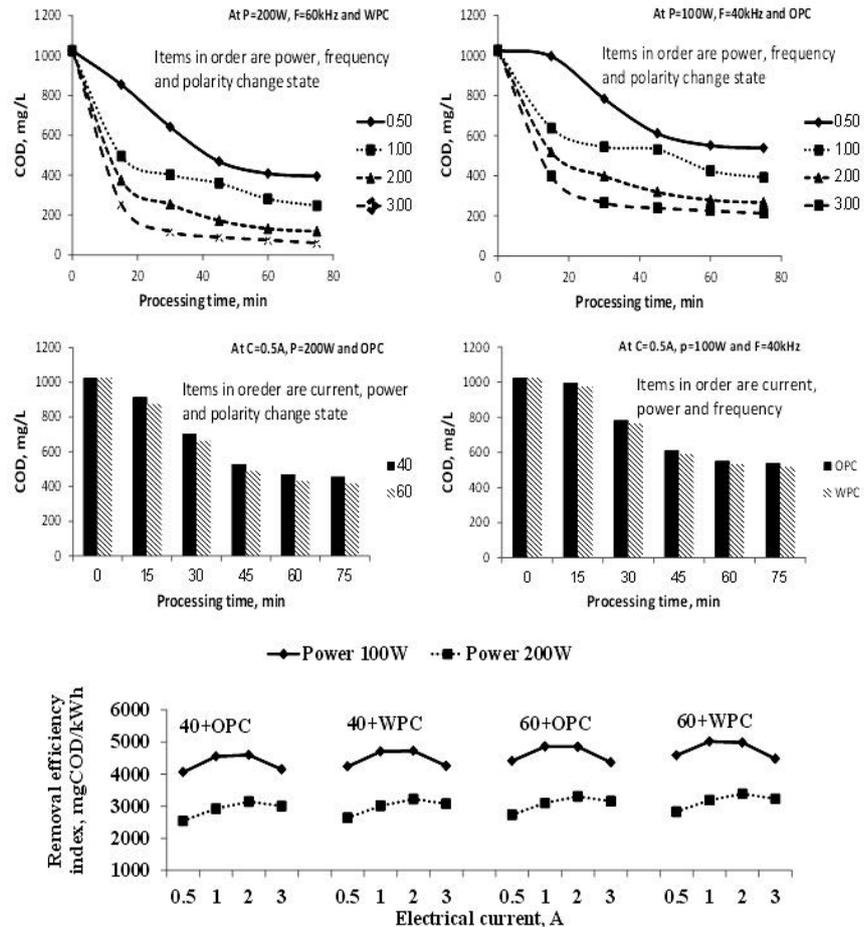
Fig. 7 The effect of electrical current, polarity changes and ultrasonic frequency on COD diminution and efficiency index at two different operating conditions of combined electro-coagulation with ultrasonication processing unit
