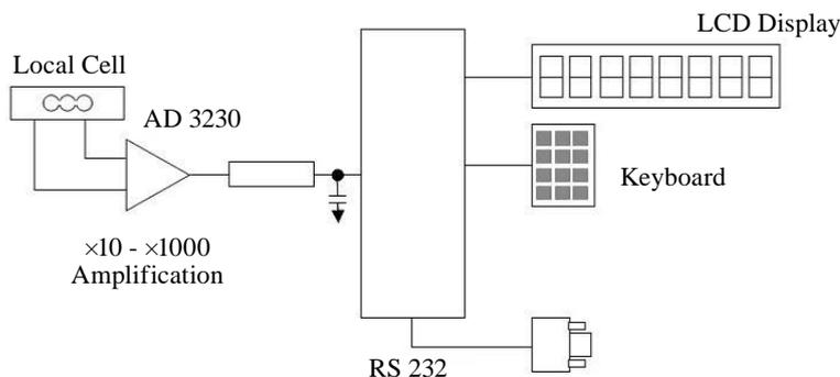
**Fig. 6** System block diagram of dynamometer
