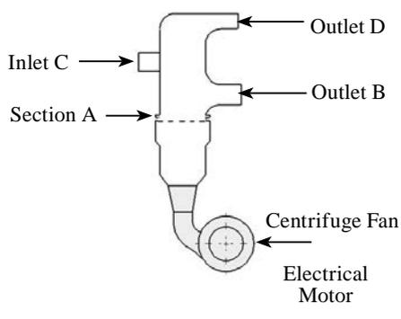
**Fig. 4** Schematic representation of the automated saffron separator, inlet and outlets of separator are shown
