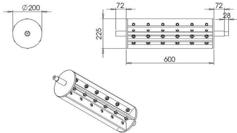
Fig. 3 Configuration of Knock-down roller
