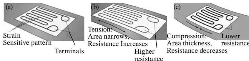
**Fig. 7** Strain gauge under different conditions (a) Normal (b) Tension (c) Compression
