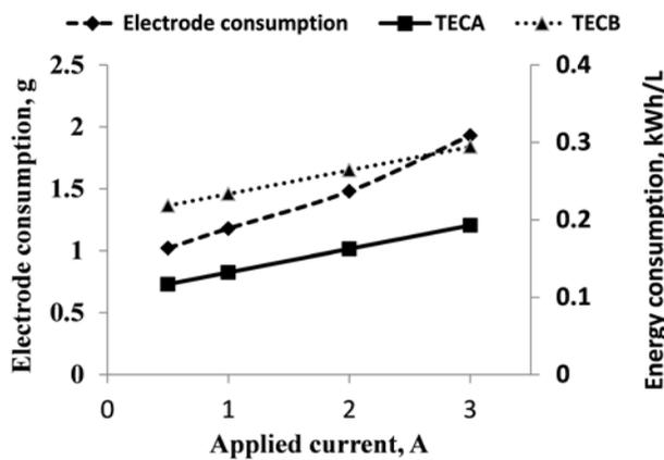
**Fig. 10** Total energy consumption of electro-coagulation with ultrasonic power level of 100W (TECA) and level of 200W (TECB) and electrode consumption during the treatment process (processing time = 75 min) under different applied currents
