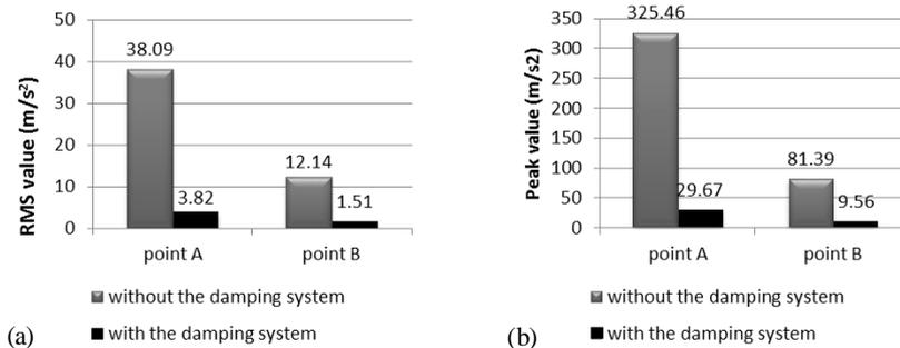
Fig. 11 RMS and peak values of the vibration signal at points A and B
