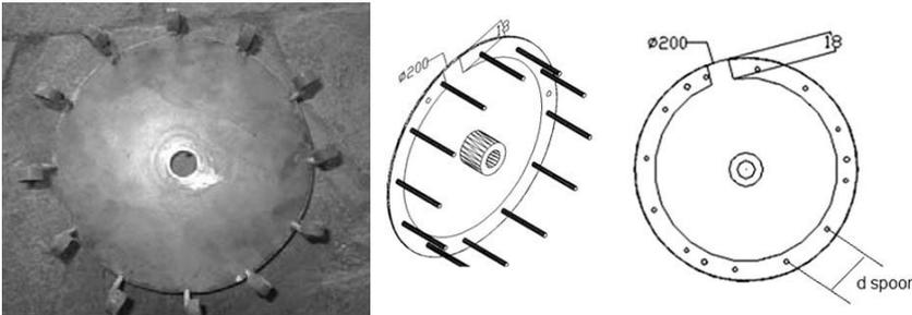
**Fig. 1** Vertical plate cup or spoon type picking metering device
