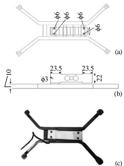
**Fig. 3** (a) Top view (b) Front view (c) Pictorial of a frame for load cell
