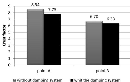
Fig. 12 Comparison of the mean of Crest factor of vibration signal at points A and B
