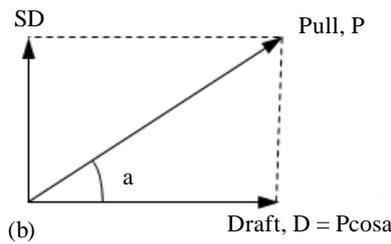
**Fig. 14** Draft measurement of (a) Push and (b) Pull type implements
