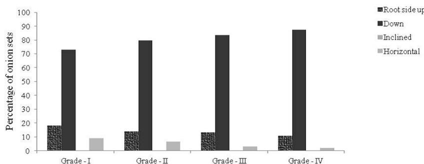
Fig. 9 Initial orientation of onion sets in the onion set metering disc for different grades
