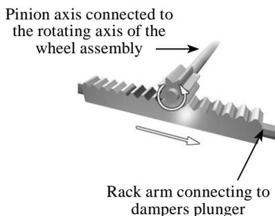
Fig. 6 Rack and pinion mechanism
