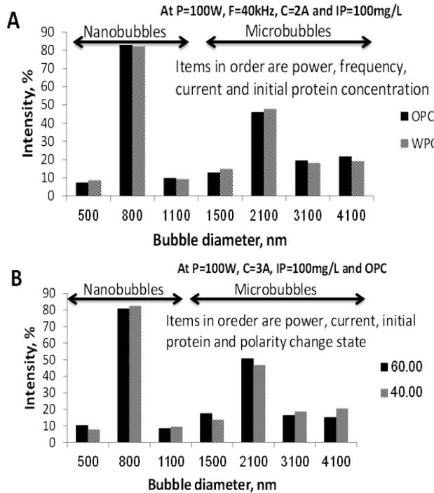
**Fig. 4** The effect of polarity change state (A) and ultrasonic frequency (B) on bubble size distribution generated as microbubbles or nanobubbles by a combined electro-coagulation with ultrasonication for bubble generator
