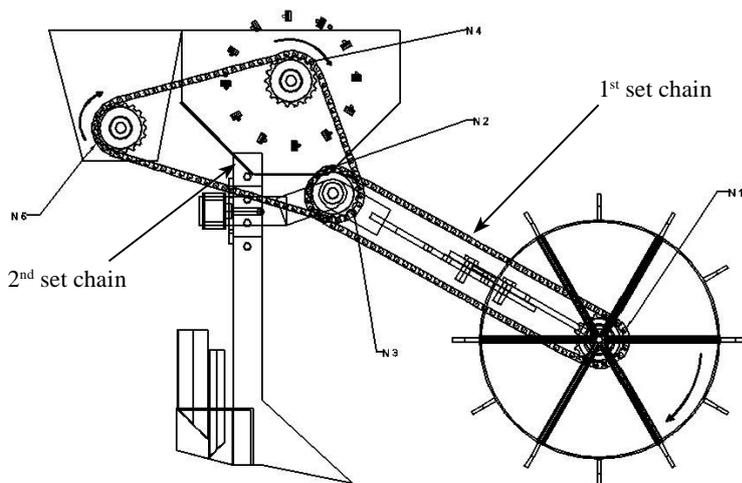
**Fig. 3** Complete driving system attached in the groundnut planter for transmission of power from ground wheel
