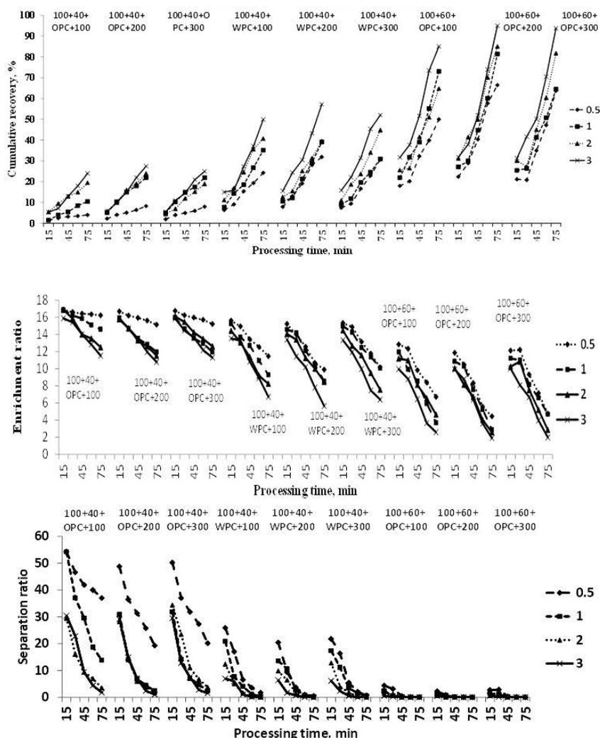
**Fig. 9** Effect of electrical current on the cumulative recovery percent and enrichment and separation ratios at different treatments; Items in order of all curves legends are ultrasonic power, W + ultrasonic frequency, kHz + polarity change state, with polarity change state WPC + or without OPC + initial protein concentration, mg/L
