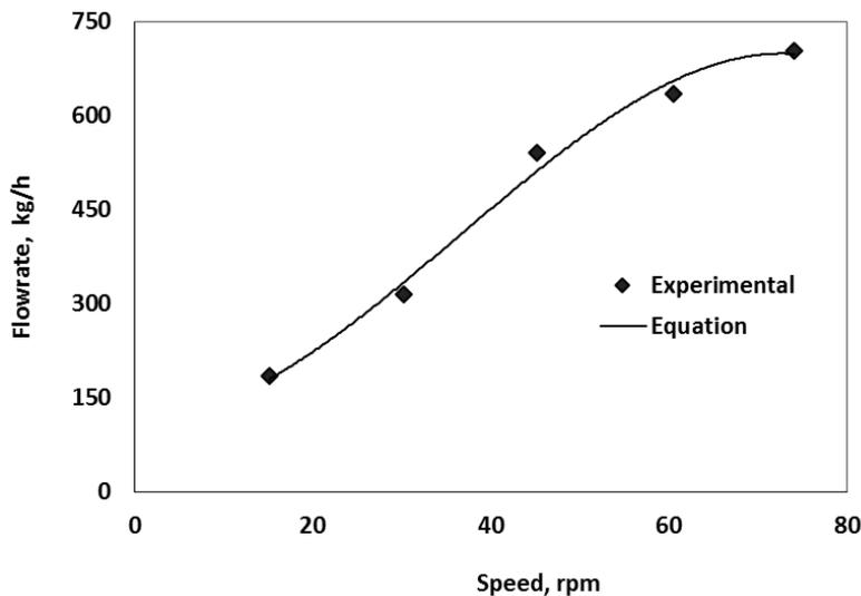
**Fig. 10** Wet mash feeding rate with speed
