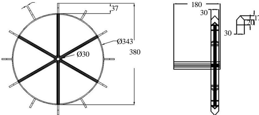
**Fig. 2** Front and side view of ground wheel for groundnut planter
