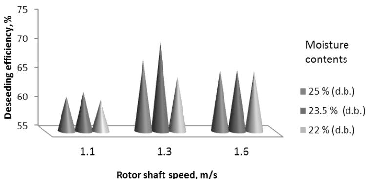
Fig. 7 Influence of moisture content, rotor shaft speed and sieve made up of bars on deseeding efficiency
