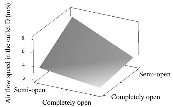
**Fig. 15** The relationship between air flow speed in the outlet D and position of outlet B and outlet D
