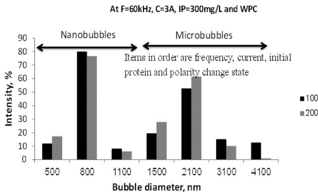
**Fig. 5** The effect of ultrasonic power on bubble size distribution generated as microbubbles or nanobubbles by a combined electro-coagulation with ultrasonication for bubble generator
