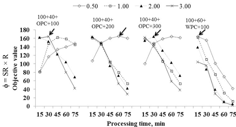
**Fig. 11** Optimal points of foam separation process under different operating conditions, arrows point the optimal point of separation process for the highest four experimental runs; Items in order for all curves legends are ultrasonic power, W + ultrasonic frequency, kHz + polarity change state, with polarity change WPC or without OPC + initial protein concentration, mg/L
