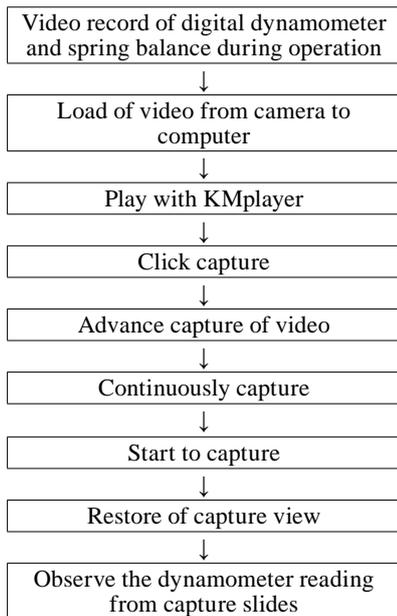
**Fig. 11** Flow diagram of data collection from video
