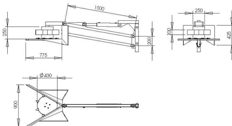
Fig. 1 Configuration of De-topper
