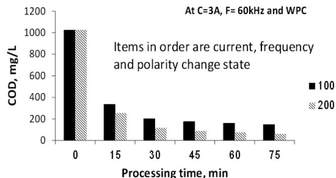
Fig. 8 The effect of ultrasonic power on COD abatement of combined electro-coagulation with ultrasonication processing unit
