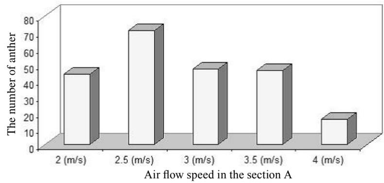
**Fig. 12** The relationship between the number of anther that remain in the section A and air flow speed in the section A
