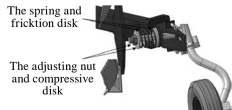
**Fig. 4** Schematic view of coulomb damper idea
