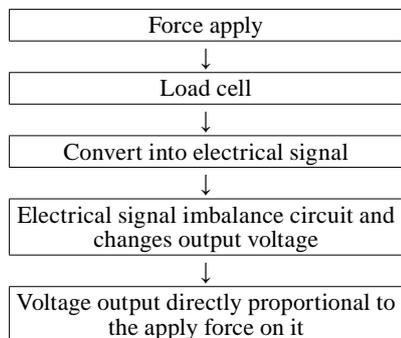
**Fig. 5** Flow diagram of the working principle of dynamometer
