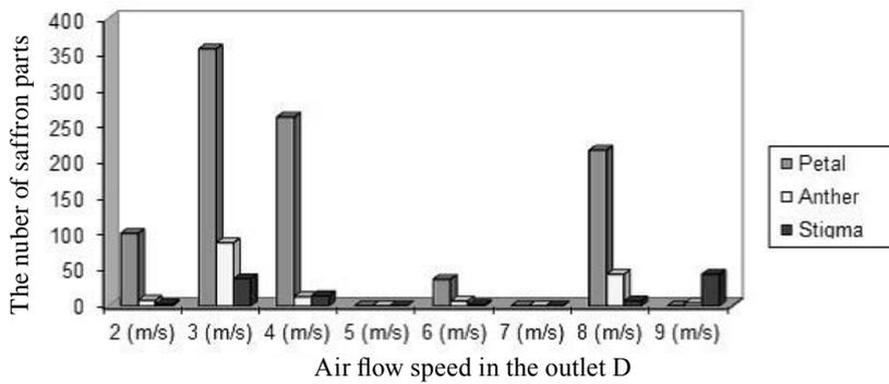
**Fig. 10** The relationship between the number of petal, anther and stigma that exit from outlet D and air flow speed in the outlet D
