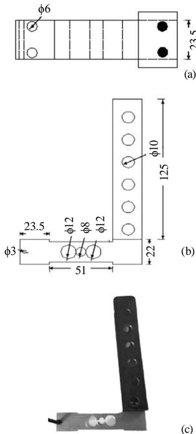
**Fig. 4** (a) Top view (b) Front view (c) Pictorial view of U-shaped frame with load cell
