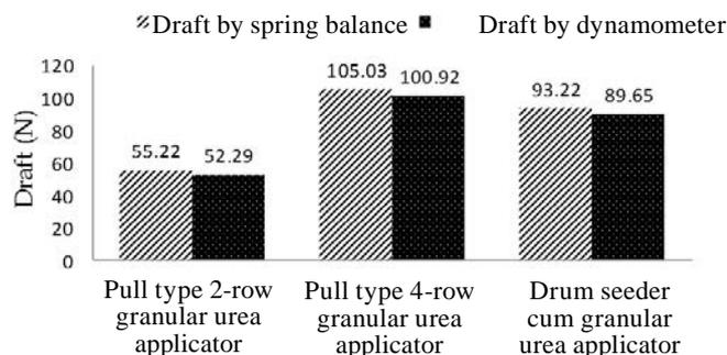
**Fig. 17** Comparison of draft of pull type implements
