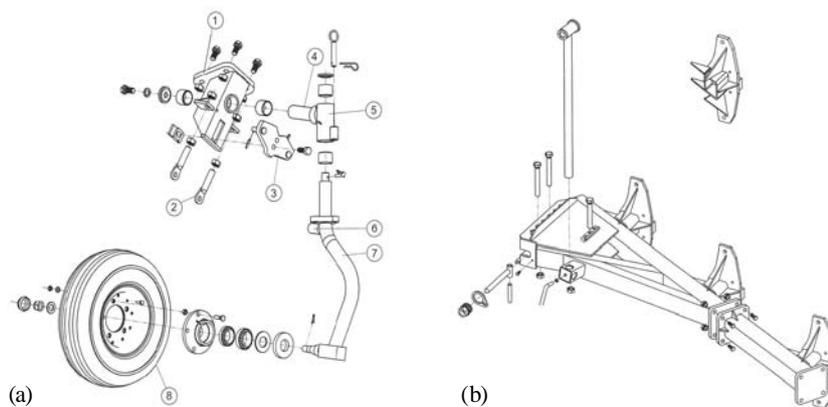
**Fig. 3** Exploded view of a) wheel assembly
