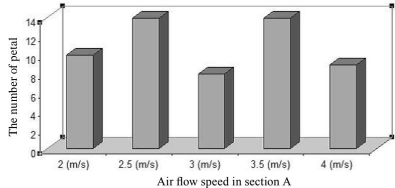
**Fig. 13** The relationship between the number of petal that remain in the section A and air flow speed in the section A
