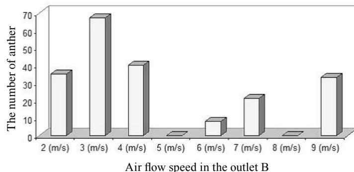
**Fig. 8** The relationship between the number of anther that exit from outlet B and air flow speed in the outlet B
