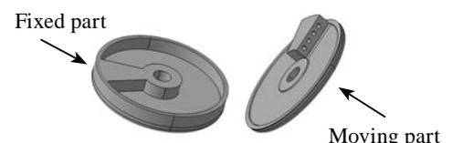
**Fig. 5** Torsional damper
