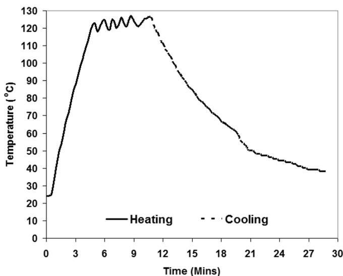
**Fig. 11** Temperature profile during heating and cooling of the dryer at the venturi throat
