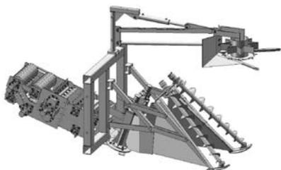
**Fig. 7** Isometric view of Solid-works model tractor operated whole cane combine harvester
