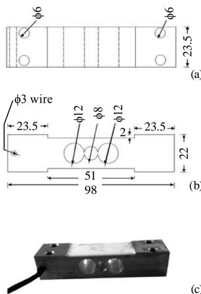
**Fig. 2** (a) Top view (b) Front view (c) Pictorial view of load cell
