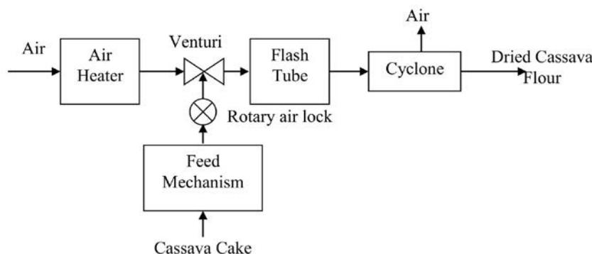
Fig. 2 Block diagram of the Flash Dryer System
