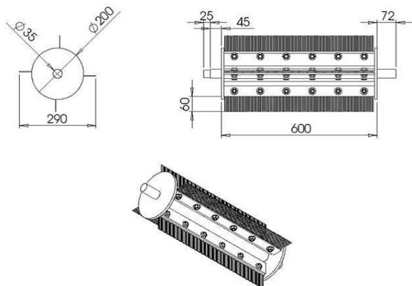
**Fig. 5** Configuration of De-trasher roller
