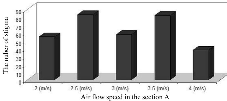
**Fig. 11** The relationship between the number of stigma that remain in the section A and air flow speed in the section A
