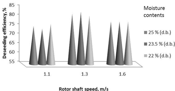
Fig. 5 Influence of moisture content, rotor shaft speed and oblong sieve on deseeding efficiency
