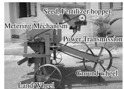
**Fig. 4** The complete view of the designed and developed groundnut planter
