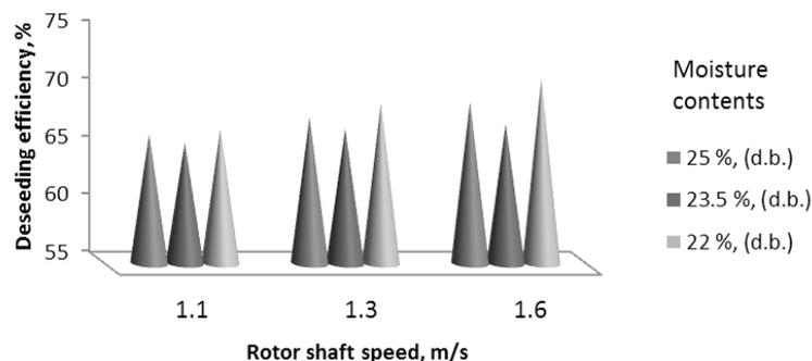
Fig. 6 Influence of moisture content, rotor shaft speed and sieve made up of rods on deseeding efficiency
