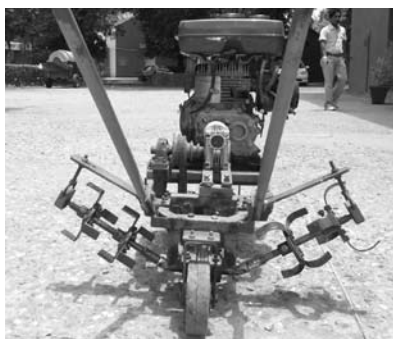
Plate 1 Developed prototype of ridge profile power weeder
