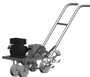
Fig. 1 Drawing of ridge profile power weeder developed in Pro-e software; c) Isometric view
