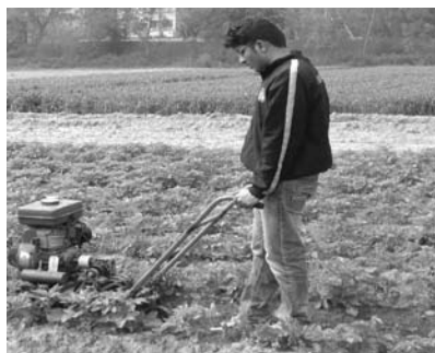
Plate 3 Field evaluation of Ridge Profile Power Weeder
