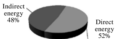
Fig. 11 Direct and indirect source of energy used in jute production
