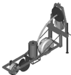
Fig. 1 Schematic view of pneumatic dibble punch planter
