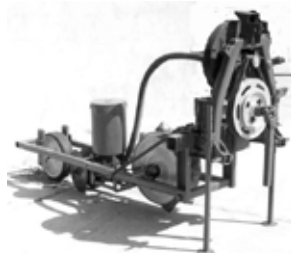
Fig. 5 The developed prototype of pneumatic dibble punch planter
