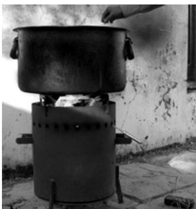
Fig. 3 Turmeric Curing with Biomass combustor
