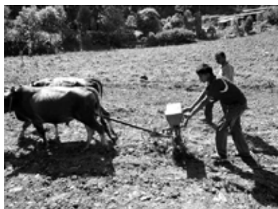
Fig. 4 Improved two row seed drill
