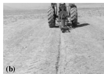
Fig. 7 The field tests (a): Planter without covering disk and press wheel and (b) Planter with covering disk and press wheel
