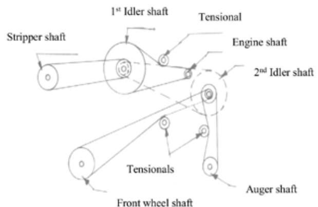
**Fig. 4b** Machine power transmission layout
