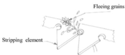
Fig. 1a Stripping operation
