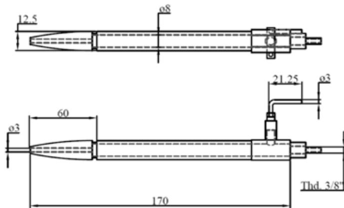
**Fig. 3** View of spoke with injector
