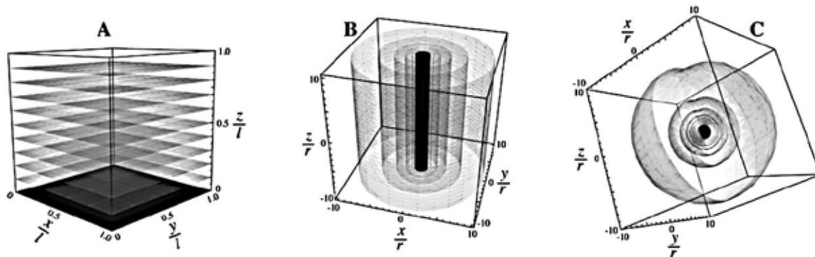
**Fig. 4** Three different diffusion bases of Fick's models used for the three geometrical shapes of Guavas (A) infinite plane model for plate slices shape; (B) finite cylinder model for cylindrical shape and (C) finite sphere model for spherical shape.
