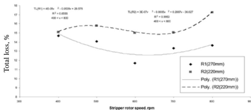
**Fig. 6** Effect of stripper rotor speed on unrecovered grains at two levels of rotor height
