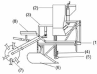
1- Main frame; 2- Seed Box; 3-Seed plate; 4- Seed tube; 5-Furrow opener; 6- Ridger; 7- Ground wheel; 8- Seat for potato dropper
