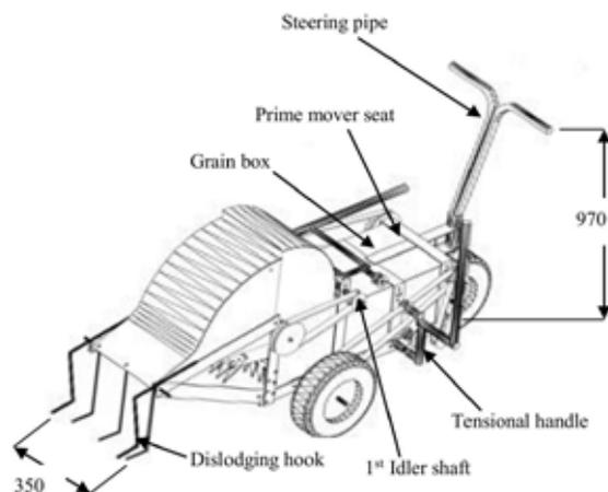
**Fig.4a** Isometric left side view of stripper harvester
