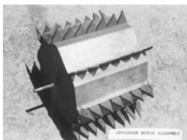
Fig. 1b Stripper rotor assembly
