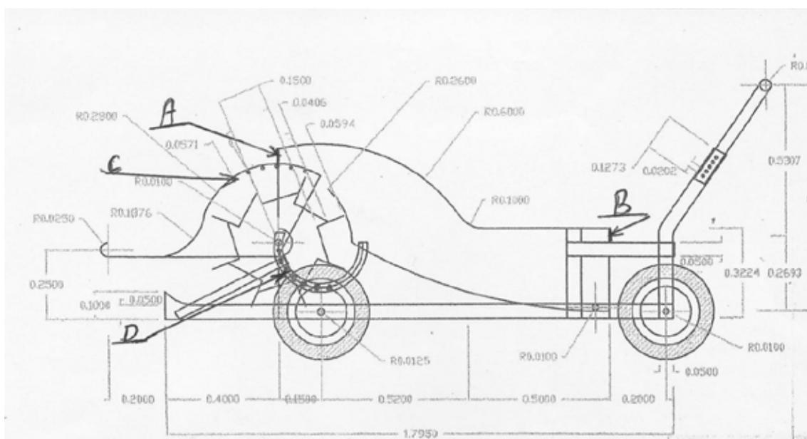
Fig. 2 Side view of stripper header.
