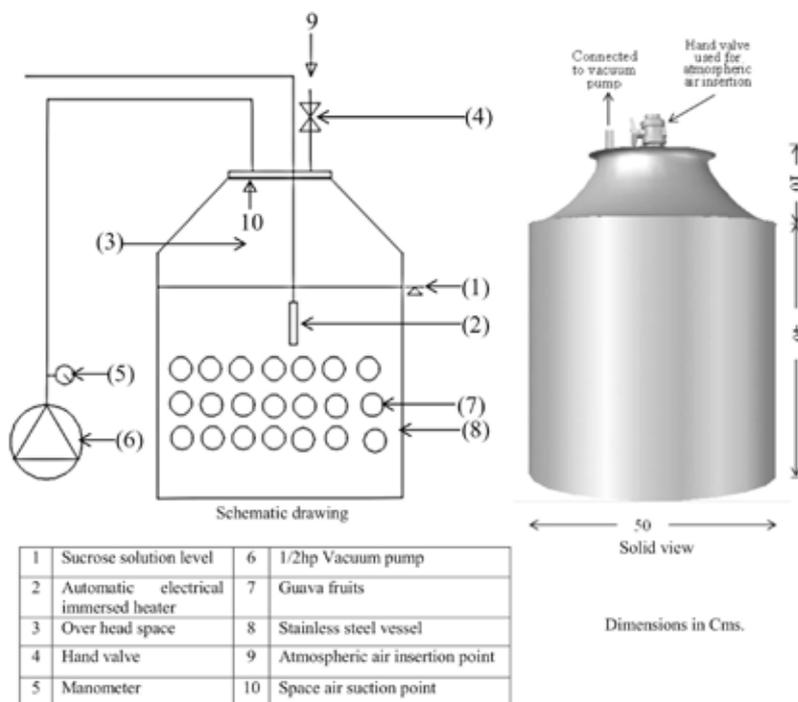
Fig. 3 Experimental setup equipped with a vacuum pulse treatment unit.
