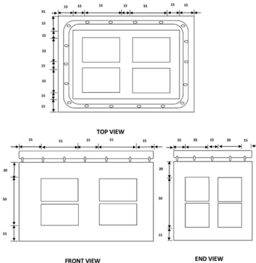
**Fig 1** Dimensions of evaporative cooling storage
