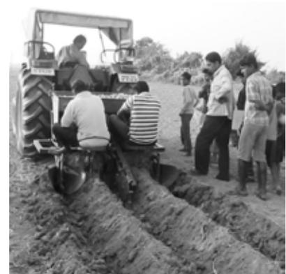
**Fig. 2** Performance evaluation of the 2-row semi-automatic potato planter
