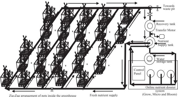
Zig-Zag arrangement of pots inside the greenhouse connected to the supply and recovery tanks in recirculation mode
