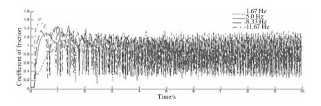
Fig. 12 Frictional characteristic curves between the rape stalk and the smooth surface at the various reciprocal frequencies
