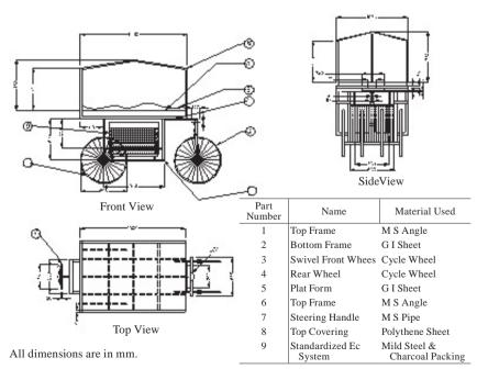
Fig. 1 Developed pushcart with EC system (Coirpith cooler)
