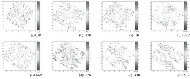
Fig. 10 The triangular layout for cumulative water distribution of sprinkler type BPXH20
