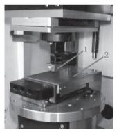
Fig. 3 UMT-2 tribometer 1. Upper frictional part 2. Bottom frictional part
