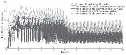
Fig. 11 Frictional characteristic curves between the rape pod shell and various surface morphologies
