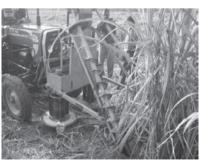
Fig. 5 IISR sugarcane harvester
