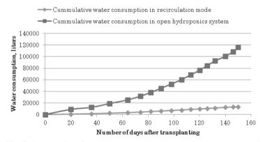
Fig. 5 Comparative of cumulative water consumption in recirculation and open system of hydroponics for 150 days period of crop cycle.
