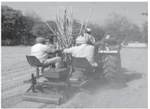
Paired row planter (PTO) Trench planter (PTO) Fig. 3 IISR developed various sugarcane cutter planters
