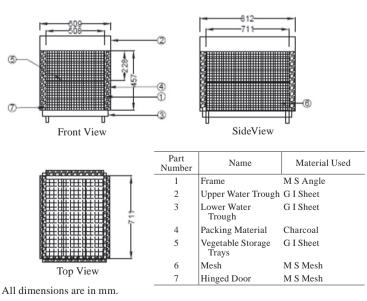
Fig. 2 Evaporative cooling system (Coirpith cooler)
