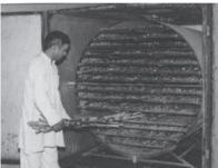
Fig. 2 IISR moist hot air treatment unit (MHAT)
