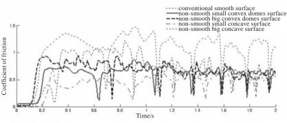
Fig. 18 The frictional characteristic curves between the rape stalk and various surficial morphology at the frequency of 8.33 Hz within 2 second
