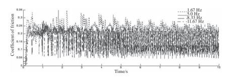
Fig. 15 Frictional characteristic curves between the rape pod shell surface and the bionic large convex dome surface at the various reciprocal frequencies
