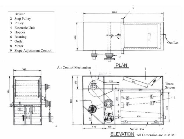
Fig. 1 Schematic diagram of the developed cumin cleaner cum grader
