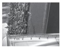
Fig. 2 The thickness of the obstructive layer on the sieve surface
