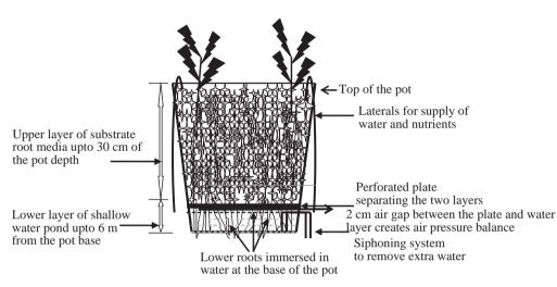
Fig. 1 Sectional view of the pot design of Hybrid Hydroponic Technology (HHT) having two layers; the upper layer of solid porous media and the lower layer of shallow water pond as separated by the perforated plate, and connected with water siphoning system.
