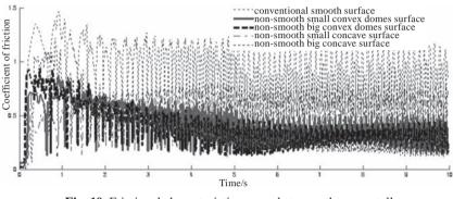
Fig. 10 Frictional characteristic curves between the rape stalk and various surface morphologies
