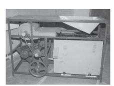
Fig. 2 Developed cumin cleaner cum grader
