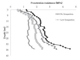
Fig. 2 Comparison the mean of penetration resistance and soil depth
