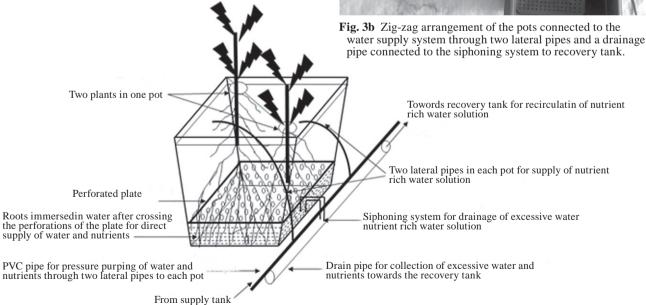
Fig. 3a Connection of the nutrient rich water supply system through the lateral pipes and siphoning system for drainage of the excessive water to the drain pipe connected to recovery tank.
