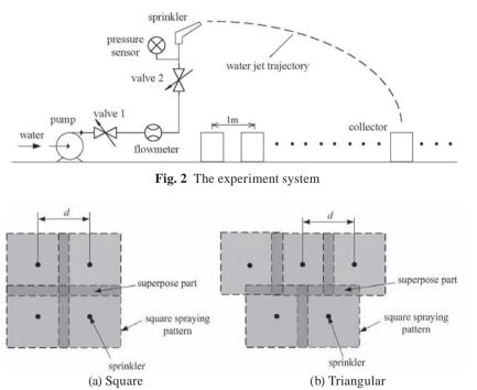
Fig. 3 Layout of the sprinklers in a square (a) and triangular pattern (b)
