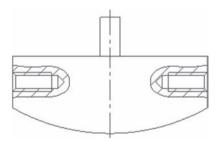
Fig. 4 Schematic of ship-shaped collet of the upper frictional part
