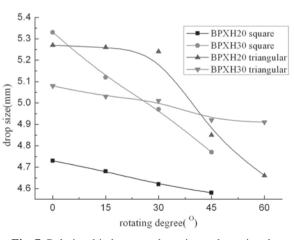
Fig. 7 Relationship between drop size and rotating degree
