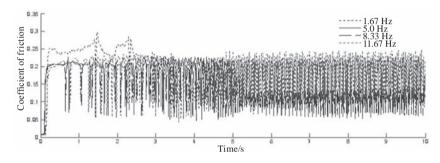
Fig. 13 Frictional characteristic curves between the rape pod shell surface and the smooth surface at the various reciprocal frequencies
