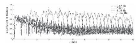
Fig. 14 Frictional characteristic curves between the rape stalk and the bionic large convex dome surface at the various reciprocal frequencies
