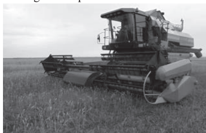
(B) on the basis of the Esil-740 harvester with a header capture of 7 m
