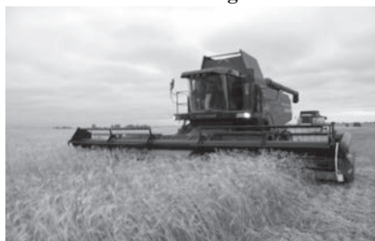
(A) on the basis of the Esil-760 harvester with a header capture of 9 m
