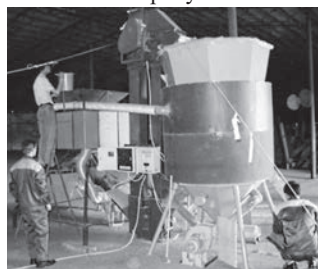
Fig. 5 Hopper microwave convective grain dryer by “AST” company
