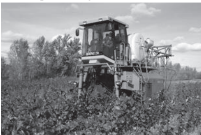
Fig. 11 A high clearance energy machine for the processing of currants
