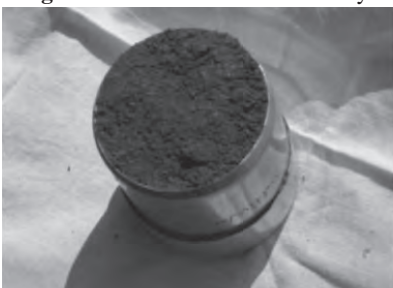
Fig. 7 Measurement of bulk density
