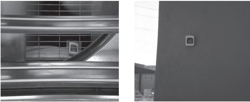
Fig. 4 Air temperature and relative humidity sensors
