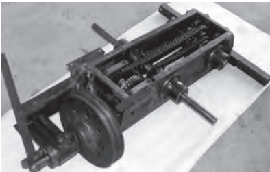
Fig. 3 A developed gearbox with a cone clutch
