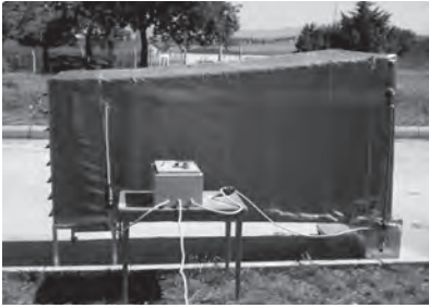
Fig. 1 Farm scale fan pad cooling unit
