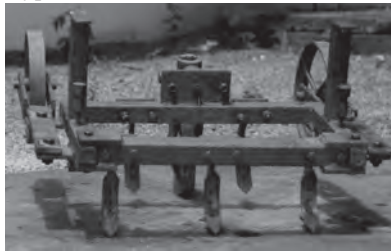
Fig. 5 Tool carrier frame with reversible type shovel
