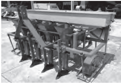
Fig. 1 Prototype of 4-row Gladiolus planter
