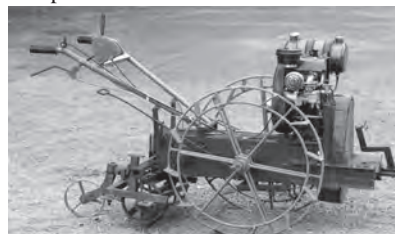
Fig. 7 Developed walking type power weeder
