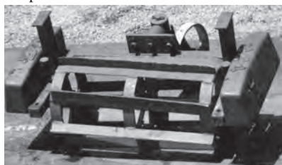
Fig. 6 View of cage roller for weeding operation
