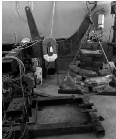
**Fig. 5** Calibration of the transducer OAE to determine vertical force constant
