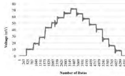
**Fig. 11** Shows the Linearity of calibration of horizontal force. The obtained equation was: Force (N) = 21.97 + 47.74 Voltage (mV)
