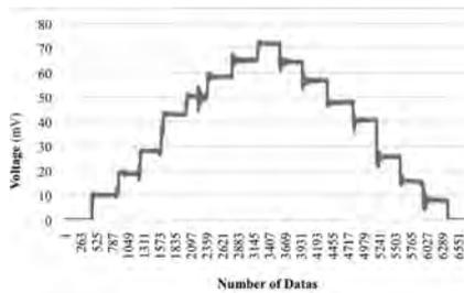
**Fig. 13** Graph showing the linearity and constant of calibration for torque transducer. Torque (Nm) = 29.34 + 0.4538 Voltage (mV)
