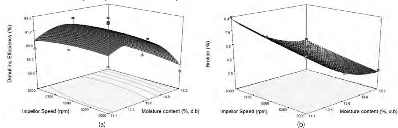
**Fig. 3a & 3b** Response surface contours for dehulling efficiency (a) and broken percentage (b) of little millet as a function of moisture content and impellor speed. For each contour plots, the third variable is fixed at ‘0’ level
