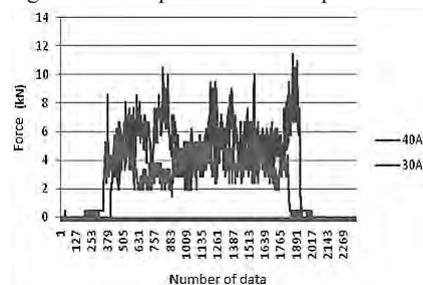
**Fig. 10** Cycles of loading and unloading of the OAE transducer during calibration with different weights for the horizontal force
