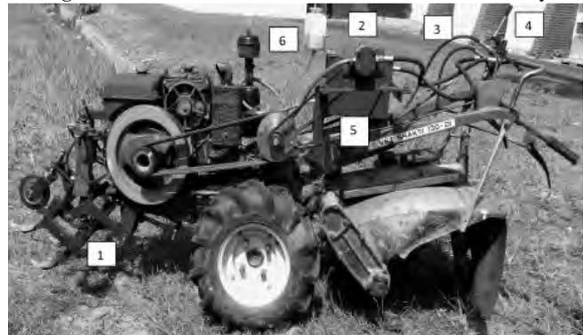
1. Front linkage system with cultivator, 2. Gear pump, 3. Pressure pipe, 4. Monoblock DCV, 5. Hydraulic oil tank, 6. Auxiliary fuel tank
