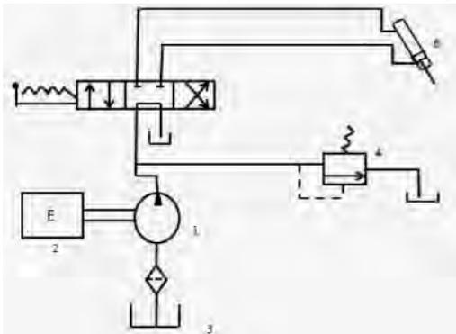
1. Pump, 2. Engine, 3. Reservoir, 4. Pressure relief valve, 5. 4/3 spring centered manually operated, DCV 6. Actuator
