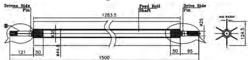
**Table 1** Specifications of spike cylinder single locking cotton feeder
