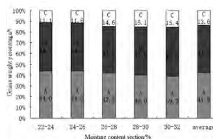
**Fig. 5** The relationship between the threshing amount of segments and the grain moisture content
