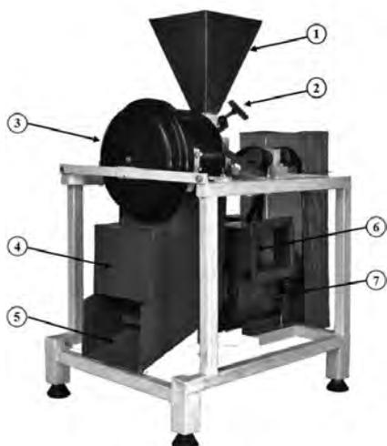
1. Hopper; 2. Feed controller; 3. Dehulling drum; 4. Husk separation chamber; 5. Rice outlet; 6. Husk outlet; 7. Belt & Pulley drive connected to motor
