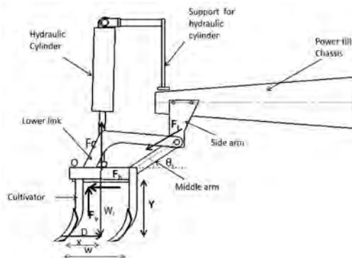
ing in the lower link in horizontal direction along the direction of motion,  $F_c$  = force acting on the hydraulic cylinder,  $W_i$  = weight of the front mounted implement,  $x$  = moment arm of resultant vertical soil and gravitational force on the implement about the lower link hitch point,  $Y$  = height of cross-shaft from centre of resistance,  $w$  = width of cultivator,  $\theta_i$  = angle of middle link with the horizontal.
