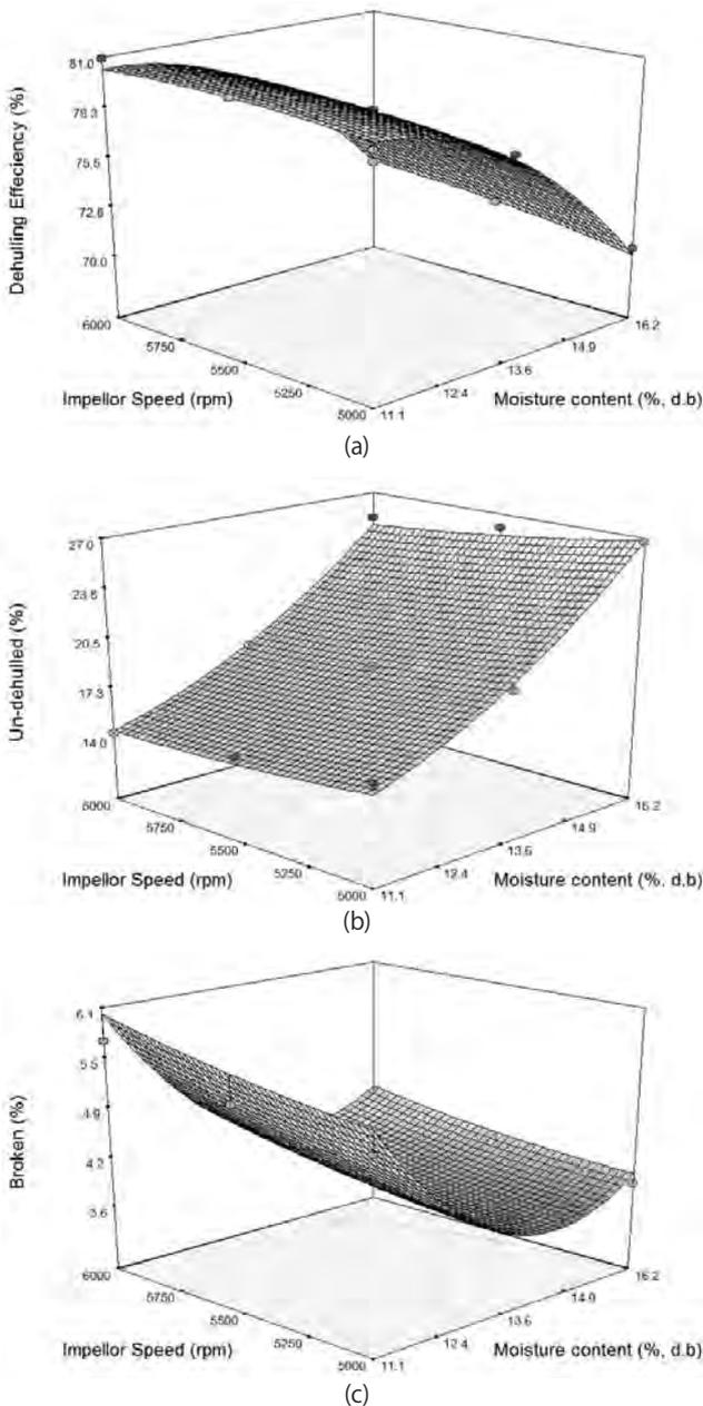
**Fig. 6a, 6b & 6c** Response surface contours for dehulling efficiency (6a), un-dehulled percentage (6b) and broken percentage (6c) of barnyard millet as a function of moisture content and impellor speed. For each contour plots, the third variable is fixed at '0' level
