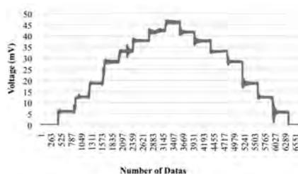
**Fig. 9** Graph showing the linearity of calibration of OAE transducer for vertical force. The obtained equation was: Force (N) = 8.073 + 75.00\* Voltage (mV)
