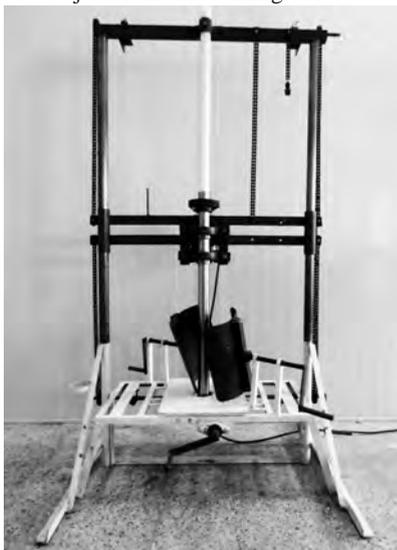
Fig. 4 Developed semi mechanised jackfruit splitting unit
