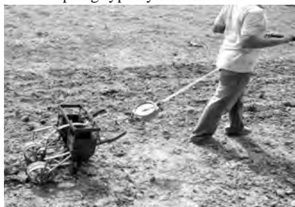
Fig. 3 Testing of check row planter
