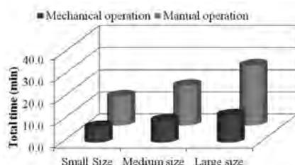
**Fig. 10** Total time taken for cutting jackfruit by mechanical and manual methods
