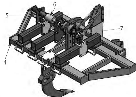
low adjustment of the frequency of oscillation from 3.3 to 4.9 Hz and amplitudes from 0.060 and 0.070 m. **Figs. 1** and **2** show the main components of the device designed and built by the Tecnomec Agrícola S. A. de C.V. Company. The apparatus is integrated by an oscillation tine (1), an oscillatory mechanism connecting rod crank (2), an extended octagonal transducer (3), structure or chassis (4), a hydraulic motor (5), a torque transducer (6) and an oscillation frequency sensor (7).
