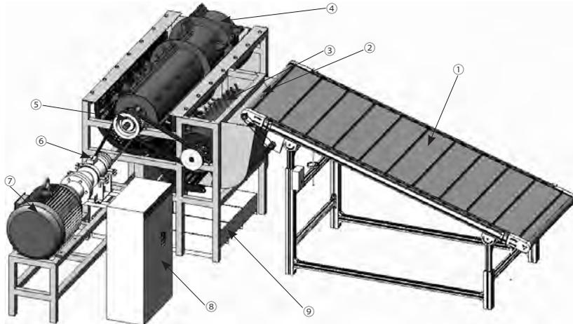
1. Feeding device, 2. Feeding port, 3. Tangential flow drum, 4. Axial flow drum, 5. Grid grating, 6. Torque speed sensor, 7. Motor, 8. Electrical control cabinet (inverter), 9. Grain collection box
