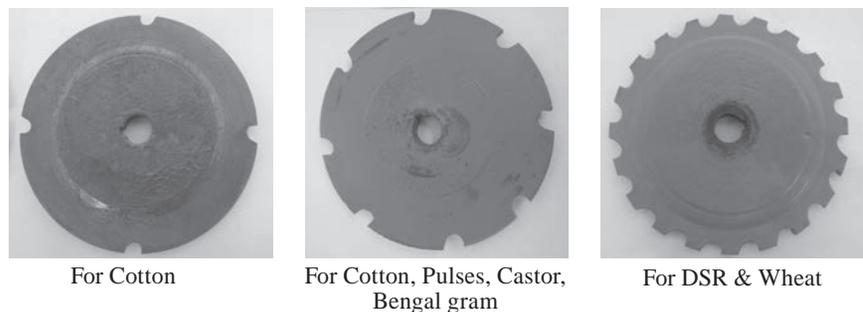
**Fig. 2** Different types of seed plates.
