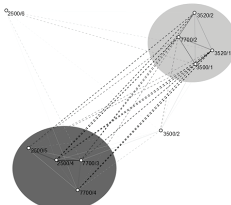
Fig. 6 An energized correlation graph of mechanical harvesters. Dark lines depict strong correlation between harvesters, while dashed lines depict negative correlation values
