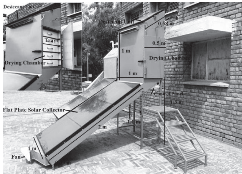
Fig. 1 Developed desiccant integrated solar dryer showing drying chamber and desiccant unit
