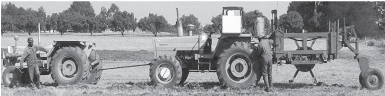
Fig. 4 Setting-up for a tillage test-run [the swivel wheel at the rear end of the rotavator tool-frame carrier was lifted off the ground during tillage experiments and the depth setting was controlled by the tractor three-point hitch system
