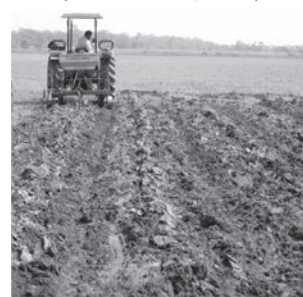
Fig. 5 Subsoiler-cum-differential rate fertilizer applicator (Thakur et al. , 2008)
