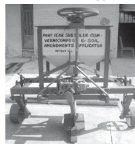
Fig. 6 Developed subsoiler-cum-vermicompost and soil amendments applicator
