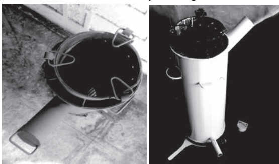
Fig. 2 Development of open top gasifier for community cooking
