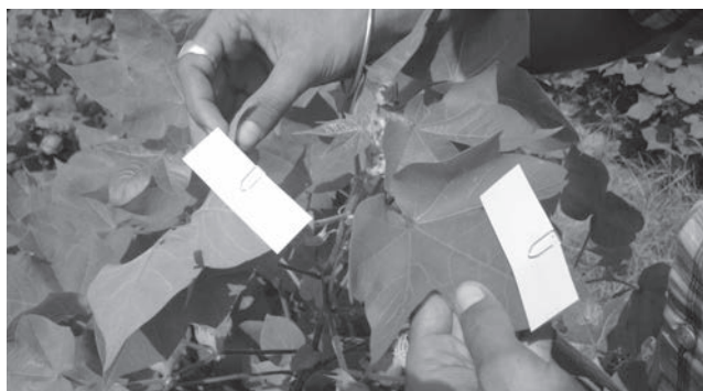
Fig. 5 A view of water sensitive paper stapled on to cotton canopy
