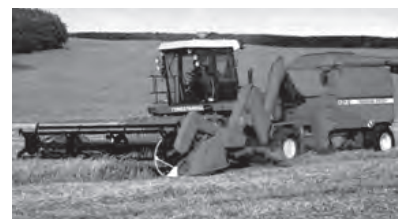
Grain harvester complex KZR-10 “Polesje” with front mounted header and axial rotary thresh dram-separator also fastened behind to UES by the block of air-cleaning with a grain bunker. - productivity on a grain up to 20 t/hr
