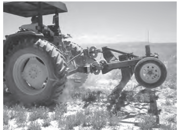
Fig. 2 Apparatus set for field evaluation, showing the integral force transducer
