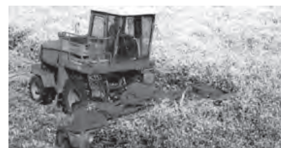
Rotary mower-crusher KPR-6 “Polesje” with demountable conditioners for crushing of grasses and stacking two swaths. - productivity up to 6 hectare/hr
