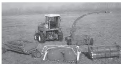
Forage harvester complex K-G-6 “Polesje” with chopper and adapters for cutting green grass, haylage and silage from grasses and corn. - productivity up to 90 t/hr
