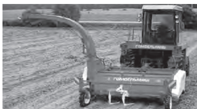
Sugar-beet harvester KSN-6 “Polesje” for one pass cuts tops, digs out, cleans and stacks Rotor”roots in a row between wheels of power unit. - productivity up to 2 hectare/hr
