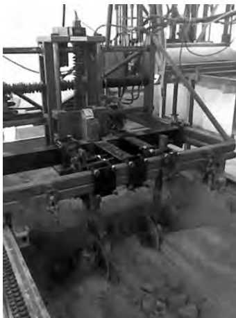
Fig. 7 Positioning coulters in front of the plowing tool for the first and second set of experiments
