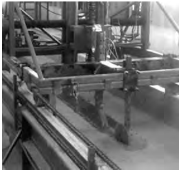
Fig. 4 Positioning coulters in front of the plowing tool for the first and second set of experiments
