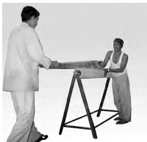
Fig. 5 Pictorial view of manual grooving of leather roller
