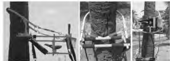
Upper and lower frame assembly fitted in palmyrah tree
