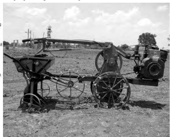
Fig. 2 Isometric view and assembled view of the self propelled garlic clove planter
