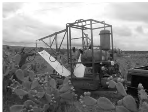
Fig. 6 Whole assembly for mechanical harvesting aid for tunas in the field
