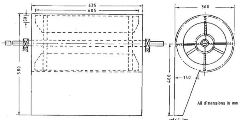
**Fig. 5** Flap roller of tractor-operated sugarcane cleaner
