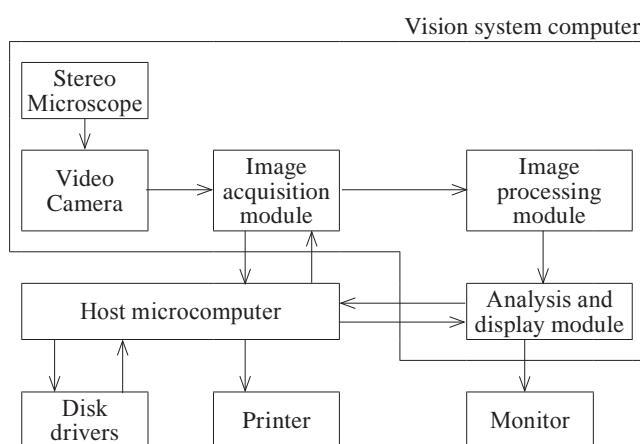
**Fig. 3** Computer vision instrument for detecting stress cracks in rice kernels
