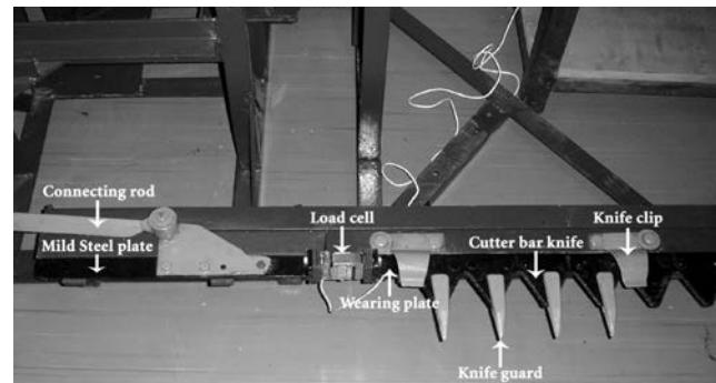
obtained by subtracting the inertial forces and frictional force of idle reciprocation from the gross dynamic cutting force. The force calculated for each position of the cutter bar was plotted as a force - distance curve as shown in **Fig. 3**. The peak cutting force (P<sub>fc</sub>) required for harvesting the selected maize fodder crops was recorded for all treatments.
