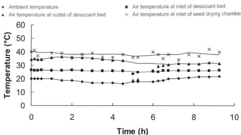
**Fig. 4** Temperature of air at inlet and outlet of desiccant bed as a function of time during regeneration of desiccant
