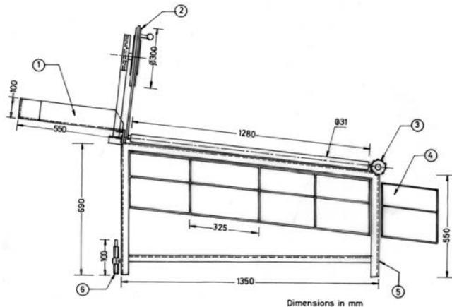
1. Feed hopper 2. Hand wheel 3. Clearness adjustment 4. Over flow
