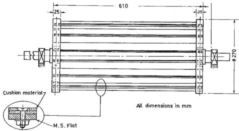
**Fig. 4** Blower of tractor-operated sugarcane cleaner
