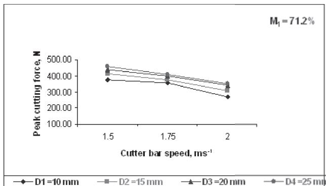
**Fig. 6** Effect of cutter bar speed on peak cutting force at selected levels of diameter and moisture content of maize stalk for 90.0 mm stroke length of cutter bar ( $L_2$ )
