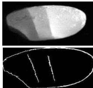
**Fig. 6** Original and processed images of a multiple stress-cracked rice
