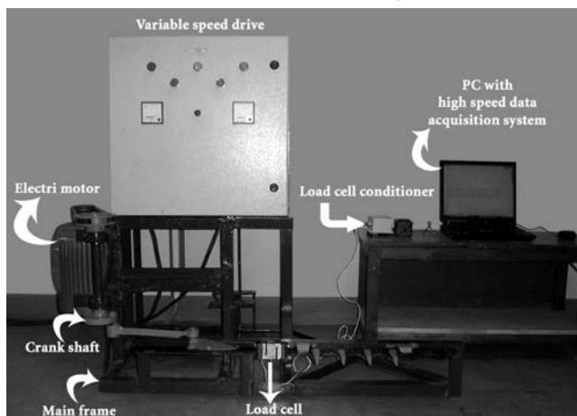
**Fig. 2** Load cell connected to wearing plate of the cutter bar
