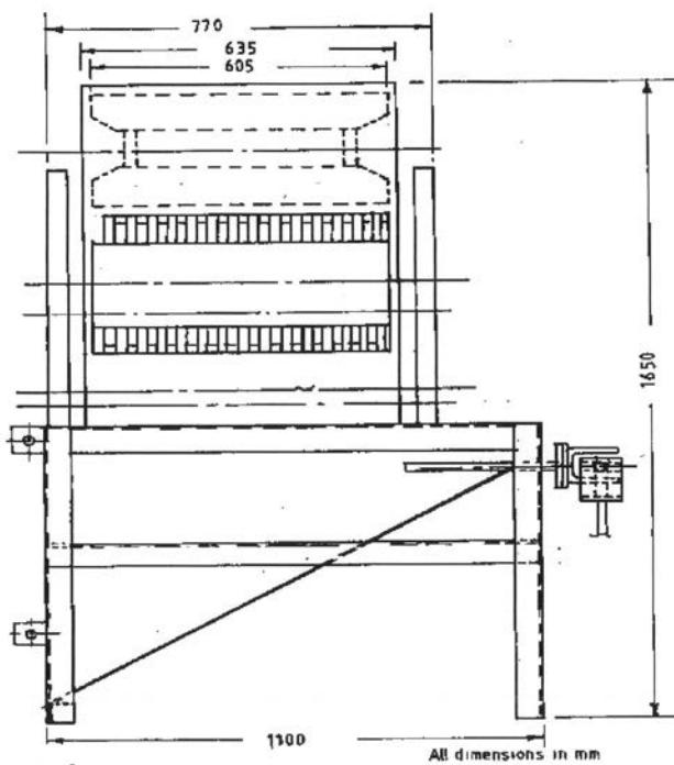
**Fig. 2** Schematic view of sugarcane cleaner (front view)
