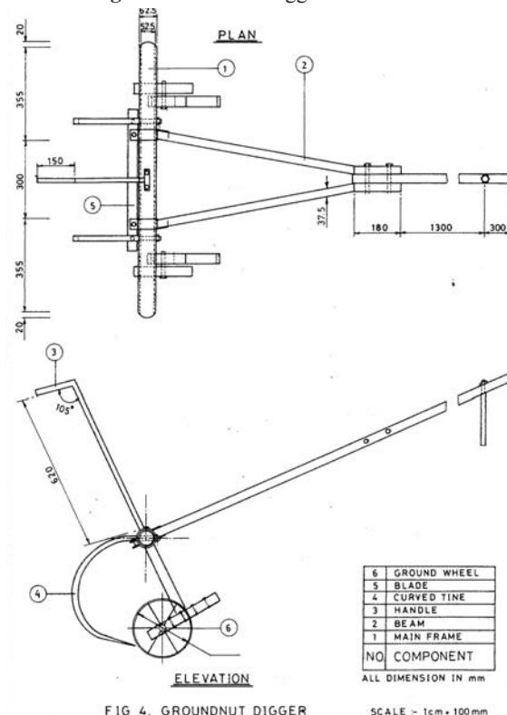
implement. For digging of groundnut, a field trial was conducted in comparison to local implements which showed encouraging results. Three tine cultivator attachments were also tested, which indicated that, when moisture was sufficient, it worked very efficiently in place of the local plough. Also, at the farmer's fields in different villages, live demonstrations were carried out and modifications were made according to the opinion of the farmers.
