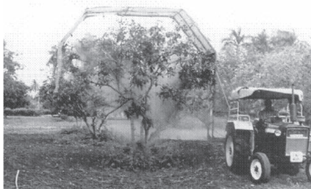
Fig. 4 Prototype parasol sprayer working in dwarf tree mango orchards
