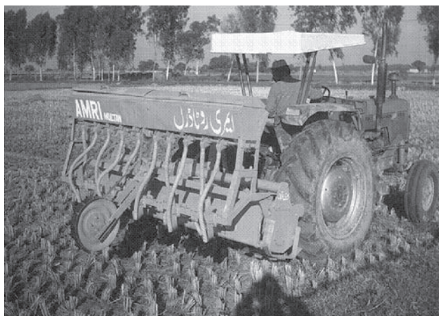
Fig. 3a Testing of rota drill in rice stubbles field
