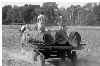
Fig. 1 Horse hitch with collar harness and standard tugs drawing the utility wagon with pneumatic rubber tires
