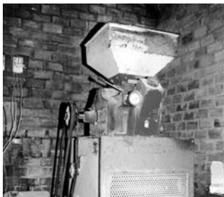
Fig. 1b Husker model HW-60A manufactured by Vinapro company-Vietnam
