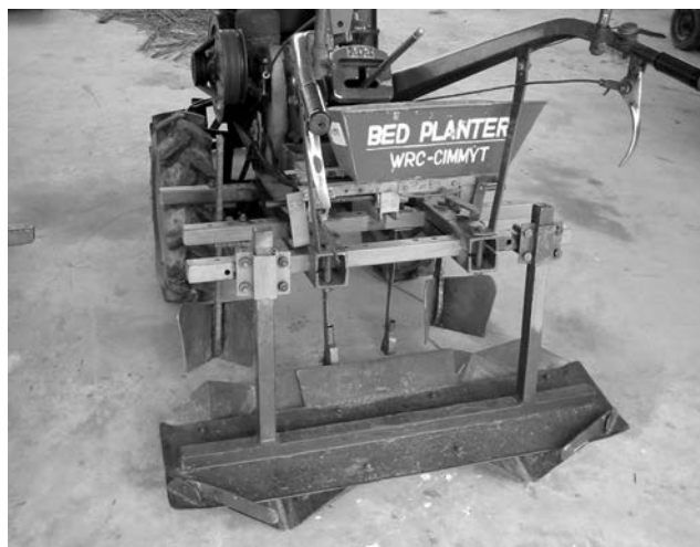
Fig. 2 Photographic view of the power tiller operated bed planter
