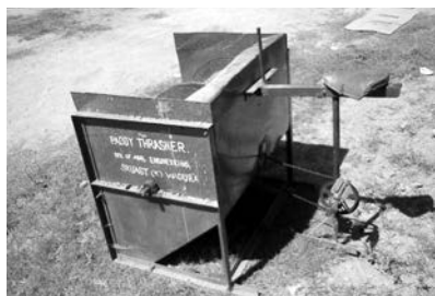
Fig. 12 Pedal operated paddy thresher in operation
