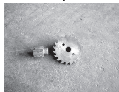
Fig. 5 Photographic view of the seed metering device
