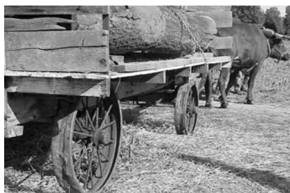
Fig. 2 Oxen with a North American-style neck yoke drawing the utility wagon with steel tires
