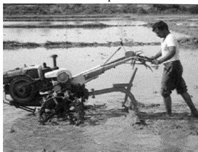
Fig. 3 Power tiller mounted wetland leveler in operation
