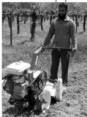
Fig. 1 Light weight power tiller in operation for seedbed preparation
