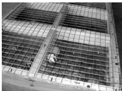
b. Bottom tray fitted with rubber balls underneath
