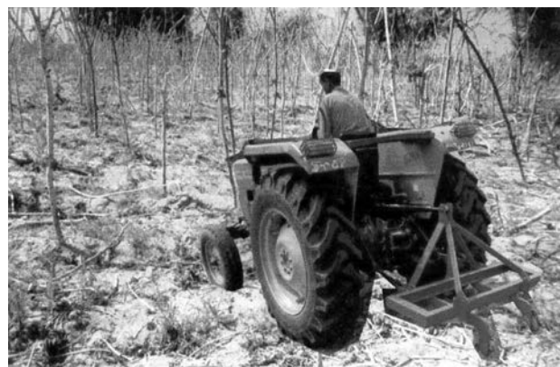
Fig. 4 Complete set of designed castor stalk uprooter
