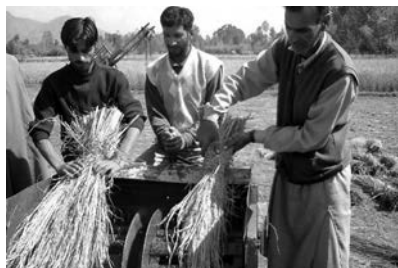
Fig. 12 Pedal operated paddy thresher in operation
