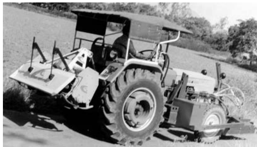
Fig. 1 Tractor operated cotton stalk shredder cum insitu applicator
