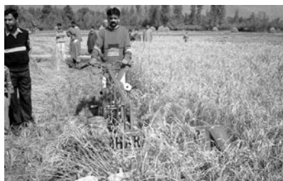
Fig. 10 Self-propelled vertical conveyor reaper in operation
