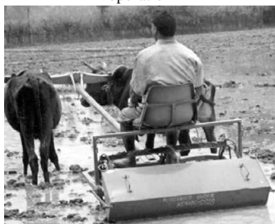
Fig. 3 Power tiller mounted wetland leveler in operation
