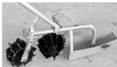
Fig. 7 Manually operated cono weeder in operation
