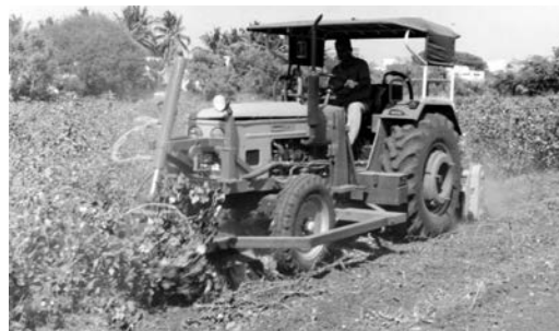
Fig. 2 Operational view of tractor operated cotton stalk shredder cum insitu applicator
