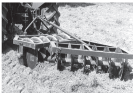
Fig. 2 View of tractor operated offset disc harrow (six discs) in operation
