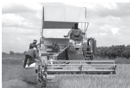
Fig. 1 Thai-designed rice combine harvester during field operation
