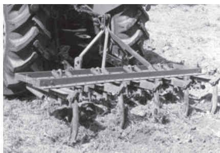
Fig. 1 View of tractor operated cultivator (nine tines) in operation
