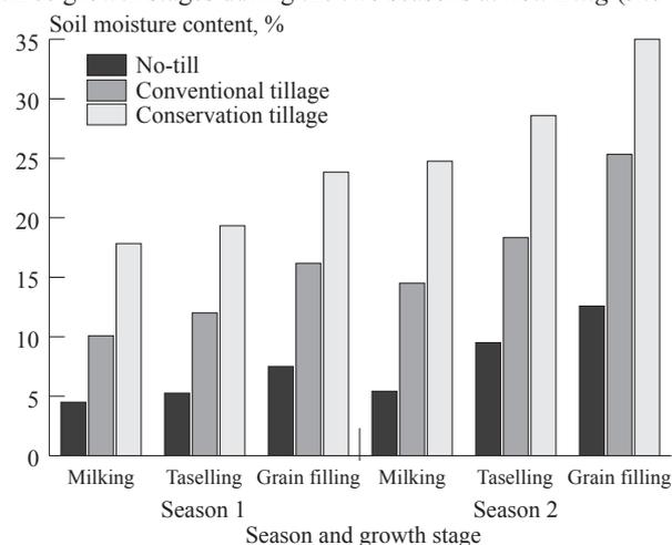
**Fig. 2** Soil moisture content (%) as affected by tillage system at three growth stages during the two seasons at *Alwan* (site 2)
