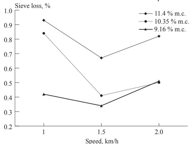
**Fig. 6** Effect of plot combine speed on total loss at different moisture contents of the crop
