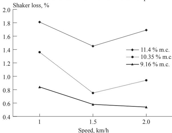
**Fig. 5** Effect of plot combine speed on sieve loss at different moisture contents of the crop
