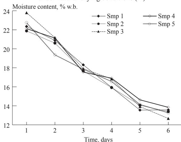
**Fig. 4** Moisture reduction with drying time under forced drying - first flow rate (FR1)
