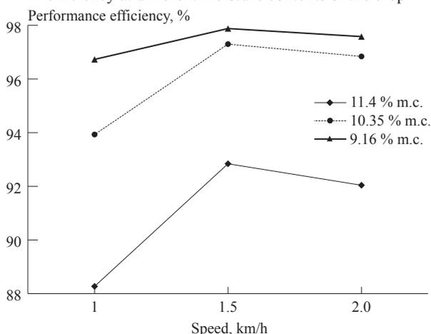
**Fig. 9** Effect of plot combine speed on threshing efficiency at different moisture contents of the crop
