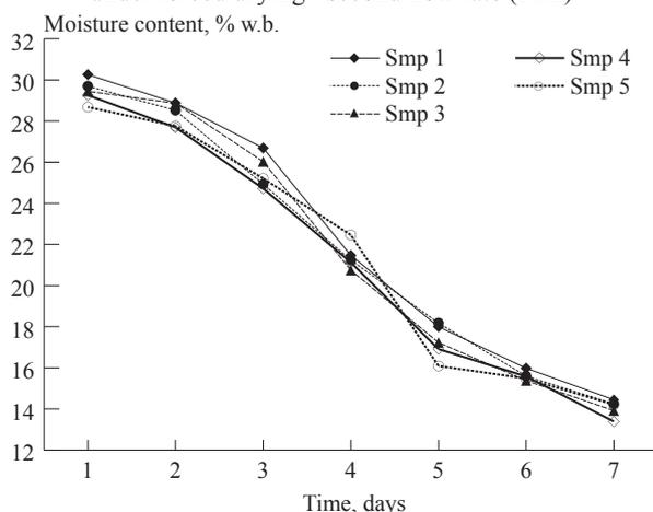
**Fig. 6** Moisture reduction with drying time for the three drying setting - average values of all samples for each setting
