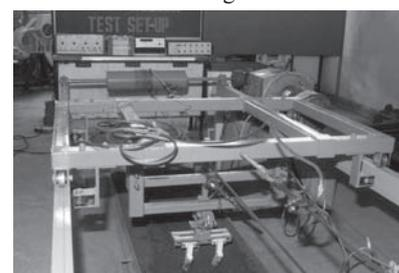
Fig. 3 Field testing of power weeder attached for optimized sweep
