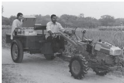
**Fig. 3** Instrumentation set up for measuring HTV of power tiller B
