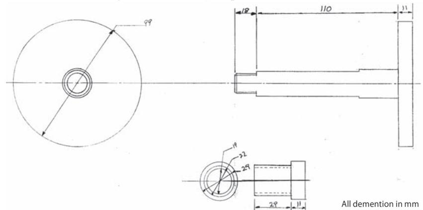
**Plate 4** The modified universal joint
