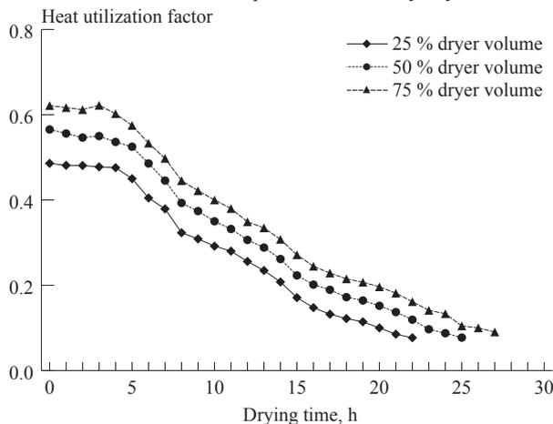
**Fig. 5** Total heat efficiency of chillies dried at 55 °C and at various capacities in a rotary dryer
