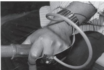
**Fig. 2** Instrumentation set up for measuring HTV of power tiller A
