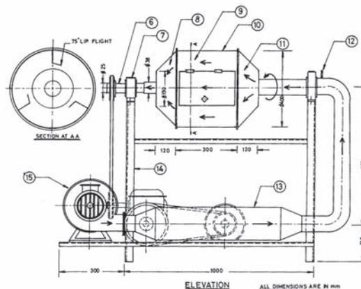
1. Reduction gear box, 2. Motor, 3. Hollow shaft, 4. Heating coil, 5. Insulator, 6. Exhaust pipe, 7. Bearing, 8. Exhaust chamber, 9. Drying chamber, 10. Rotary drum, 11. Plenum chamber, 12. Thermocouple, 13. Heating chamber, 14. Main frame, 15. Blower
