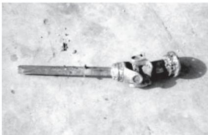
**Plate 5** Shaft assembly for power transmission
